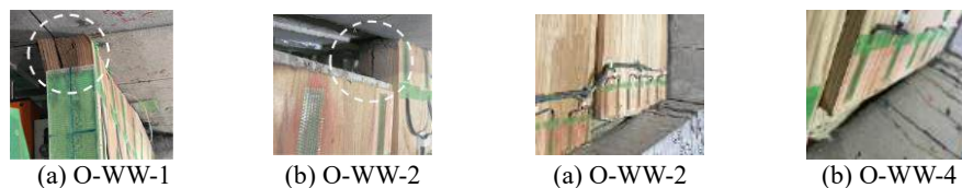
Fig.8 Out-of-plane displacement of CLT panels
