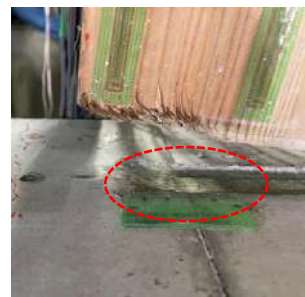
Fig.10 Failure state of embedded portion
