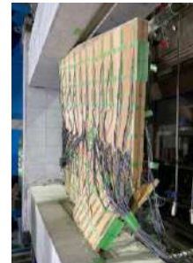
Fig.11 Final damage status of CLT panel (O-MW-1.14)
