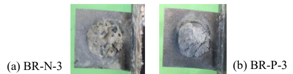
Fig. 7 Examples of deformed shape of shear connectors at end of loading
