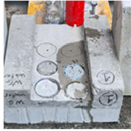
Fig.2 Coring for bond strength test
