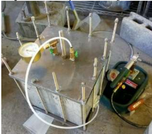
Fig.9 Water pressure test system
