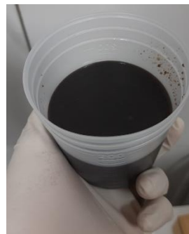
Fig.1 Prepared oil in alkali activator solution emulsion with GO as Pickering particles
