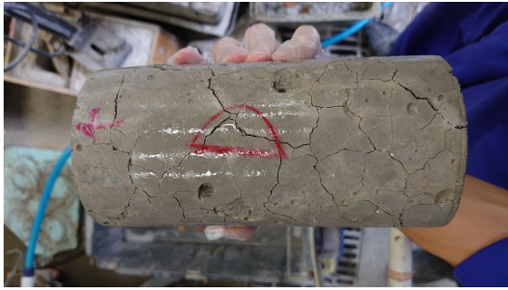
Fig.9 Crack pattern of DEF-2
