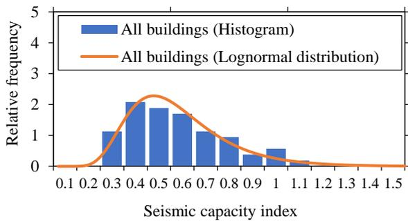
Fig.9 Seismic capacity index of investigated buildings in the Taiwan EQ
