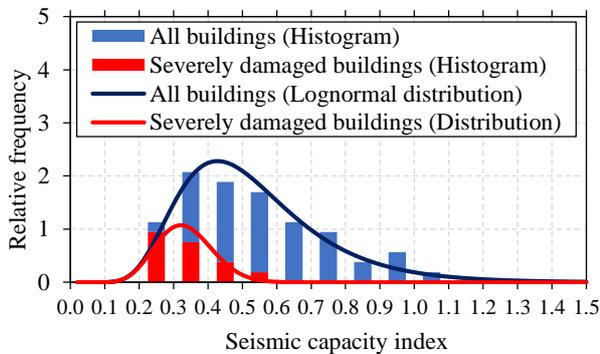
Fig.10 Distribution of seismic capacity index for total buildings and damaged buildings in Taiwan EQ
