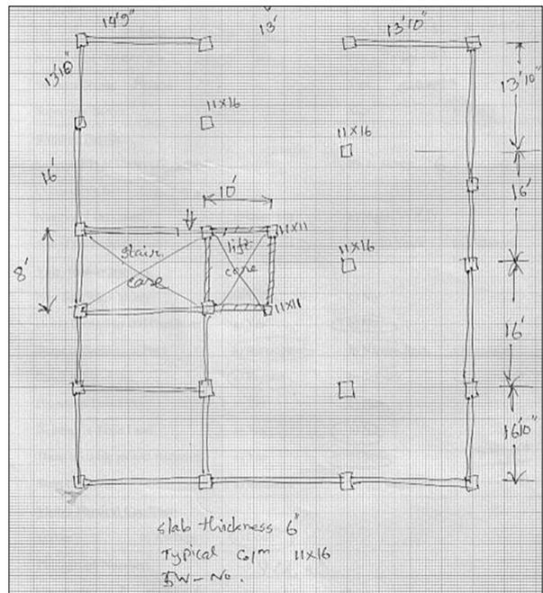
Fig.12 A typical as-built drawing for ground floor plan of building [7]
