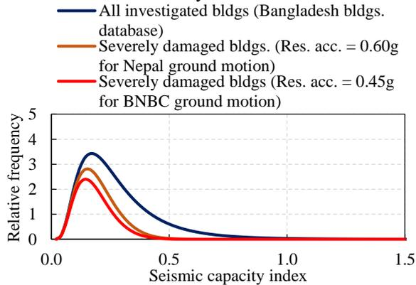
Fig.17 Distribution of seismic capacity index for severely damaged RC buildings
