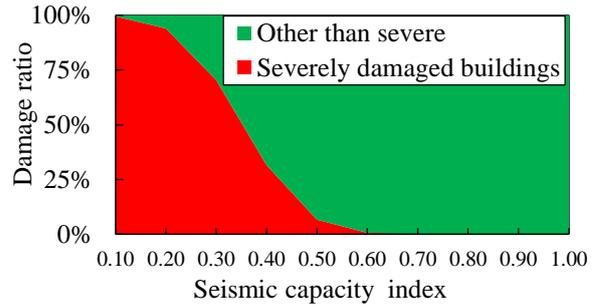
Fig.5 Correlation the seismic capacity with damage ratio based on investigated buildings
