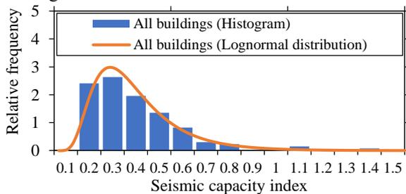
Fig. 3 Seismic capacity index of investigated buildings in the 2015 Nepal EQ
