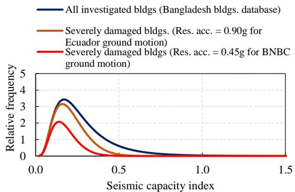
Fig. 20 Distribution of seismic capacity index for severely damaged RC building
