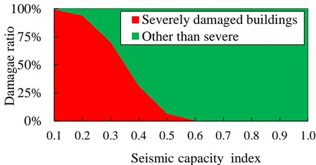
Fig.11 Correlation the seismic capacity with damage ratio based on investigated buildings
