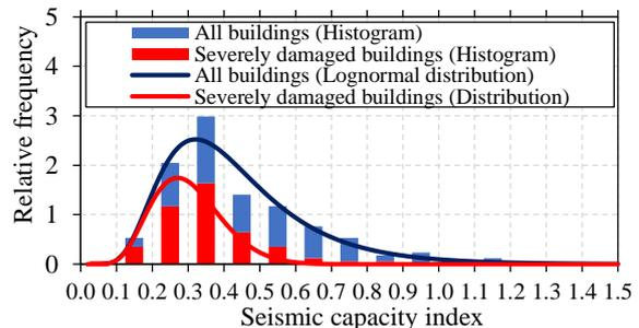
Fig. 7 Distribution of seismic capacity index for total buildings and damaged building in the Ecuador EQ
