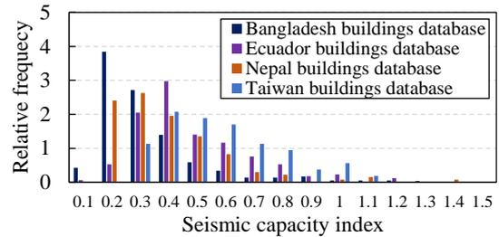
Fig. 15 Distribution of seismic capacity index of investigated buildings
