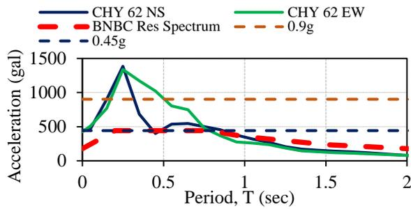
Fig. 22 Comparison of different levels of response acceleration
