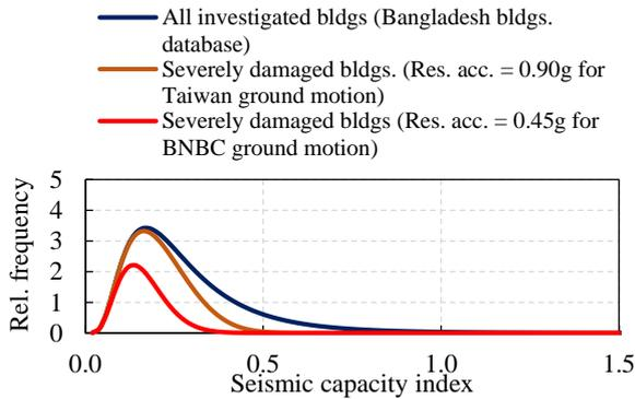
Fig. 23 Distribution of seismic capacity index for severely damaged RC building.
