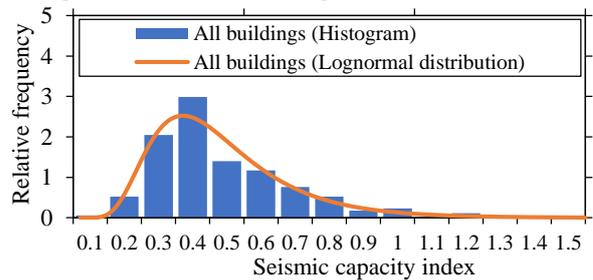
Fig. 6 Seismic capacity index of investigated buildings in the 2016 Ecuador EQ
