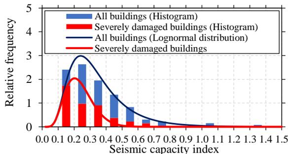
Fig. 4 Distribution of seismic capacity index for total buildings and damaged buildings in the Nepal EQ.
