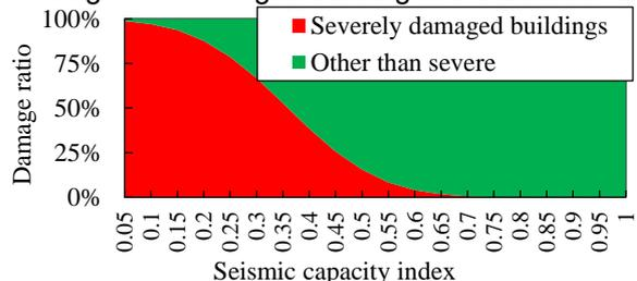
Fig. 8 Correlation the seismic capacity with damage ratio based on investigated buildings.
