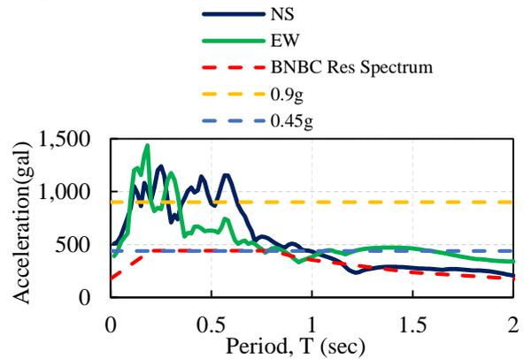
Fig. 19 Comparison of different levels of response acceleration
