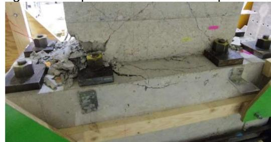
Fig.6 Damage at beam-wall joint (specimen W15 at the loading cycle of 4%)
