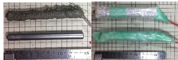
Fig.4 Steel coating and curing - Series 2
