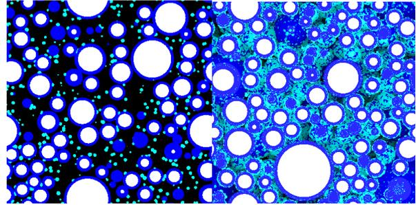
Fig.5 A two-dimensional slice of homogenous (left) and heterogenous case (right), with hydration degree=0.72
