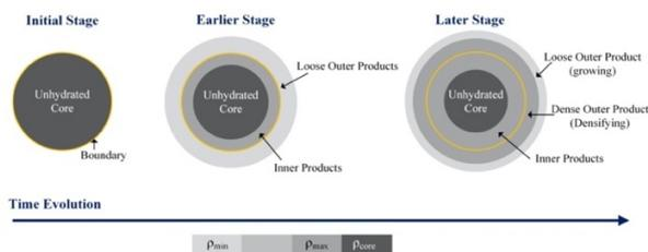
Fig. 9 Schematic diagram of simulated densification
