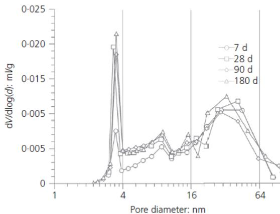
Fig.12. Derivative plot of porosity of cement paste ( $w/c=0.5$ ) tested in Nitrogen Adsorption Test [14].
