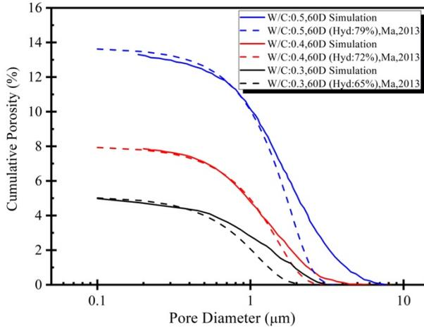
Fig.10 Computed pore size distribution with varied w/c using densification model (Age=60 Days)
