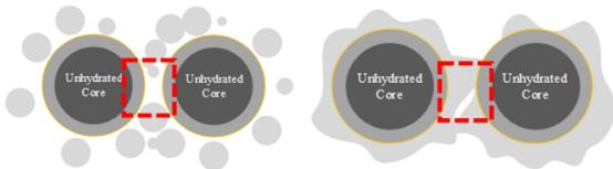
Fig.8 (a) Schematic Diagram of particle impingement in homogenous case and (b) heterogenous case
