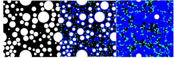
Fig.1 Homogenous Nucleation of Outer Products (Hydration Degree: 0, 0.72 and 0.85)
