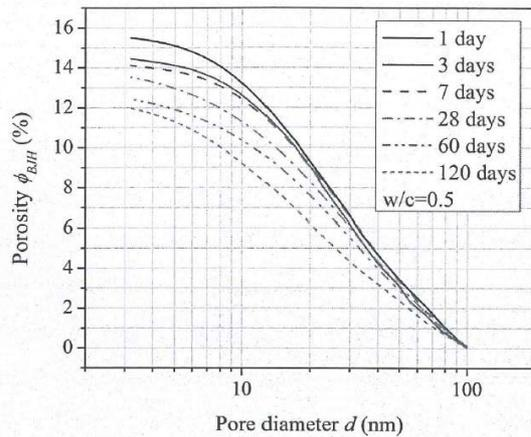
Fig.11. Porosity of cement paste ( $w/c=0.5$ ) tested in Nitrogen Adsorption Test [5].
