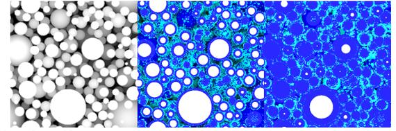
Fig.2 Heterogenous Nucleation of Outer Products (Hydration Degree: 0, 0.72 and 0.85)
