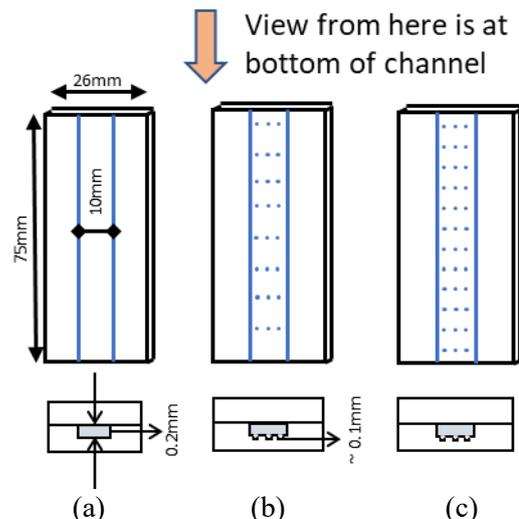
Fig. 1: Glass micro channels with variation in the number of crevices (a) No crevice (b) 27 Crevices (c) 54 crevices
