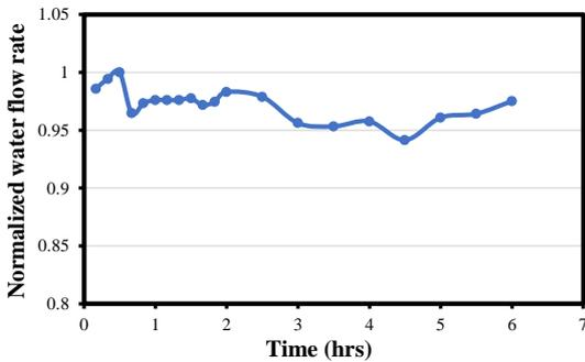
Fig. 6: Normalized water flow rate of the hydrophobic glass microchannel
