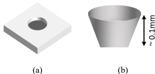
Fig. 2: (a) Schematic diagram of the crevice from top on a portion of glass plate (b) 3D view of crevice
