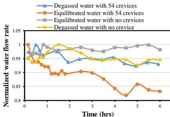
Fig. 4: Comparison of water flow test results with crevices using hydrophilic glass micro channels and with crevices
