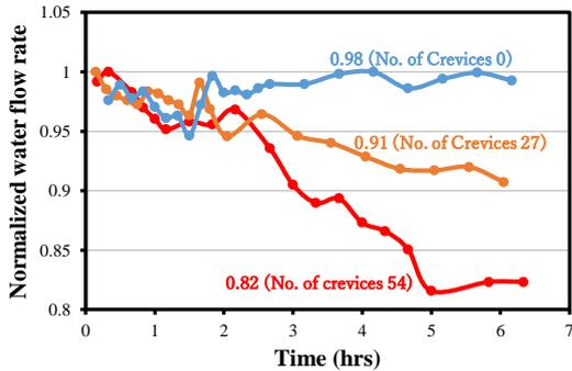
Fig. 5: Water flow rate dependency on the number of crevices present in micro channel
