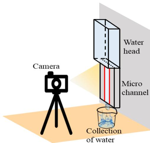
Fig. 3: Experimental set up for the water flow tests using glass microchannel
