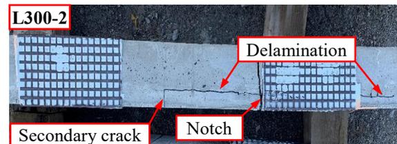
a) Side view of specimen L300-2
