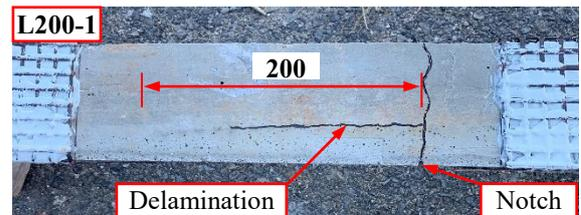
Fig.6 Delamination failure of series L200
