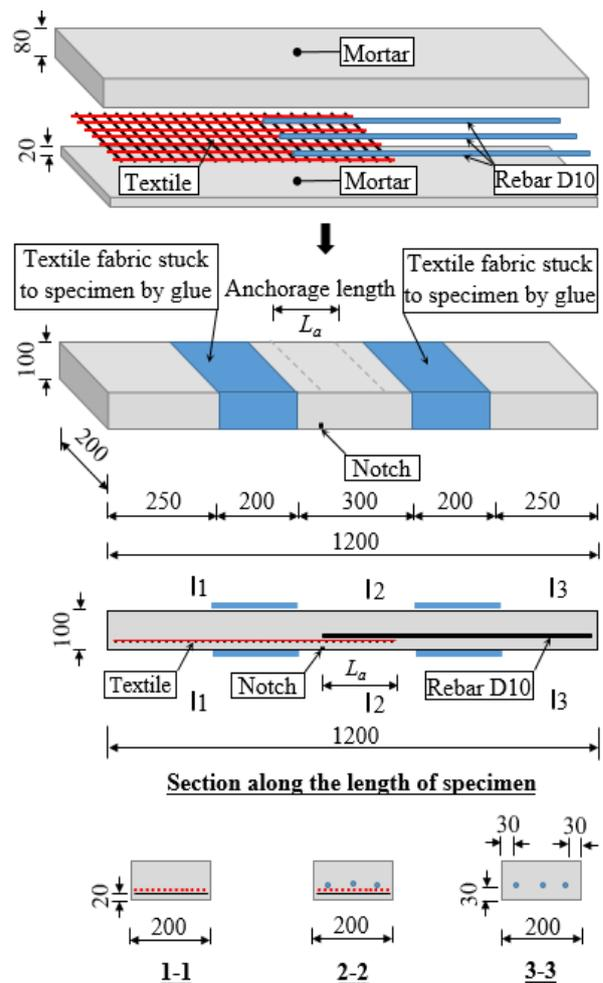
Fig.2 Sketch of specimen used for flexural test
