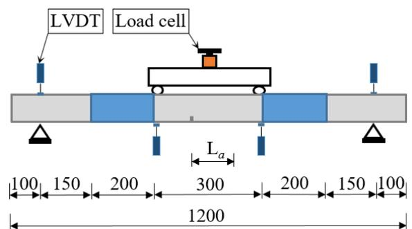
Fig.3 Sketch of test setup
