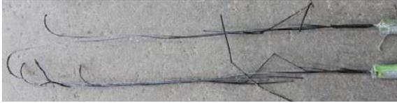
Figure 11 Failure of the hook
