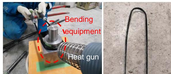
Figure 3 Bending process and a hook sample
