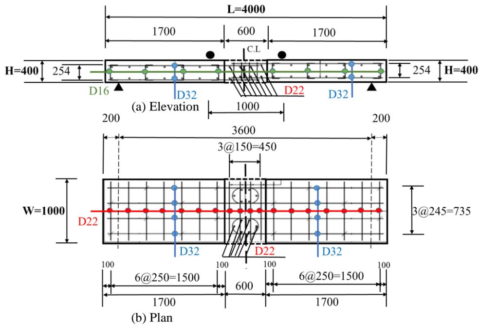
Fig. 6 Precast beams with loop joint (Case 2)
