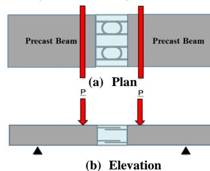
Fig. 1 Horizontal Loop Joint
