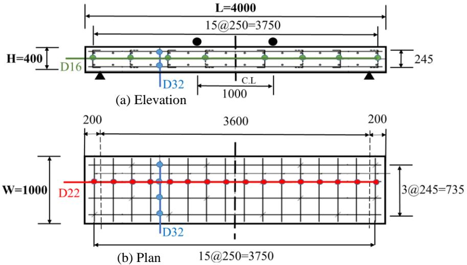
Fig. 5 Ordinary RC beam (Case 1)
