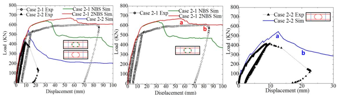
Fig. 9 Load displacement relations Case 2
