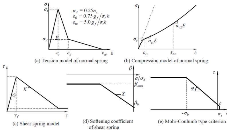
Fig. 2 Constitutive model for concrete (Yamamoto et al., 2008)
