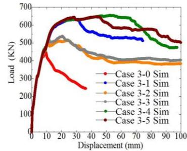
Fig. 11 Load displacement relations Case 3
