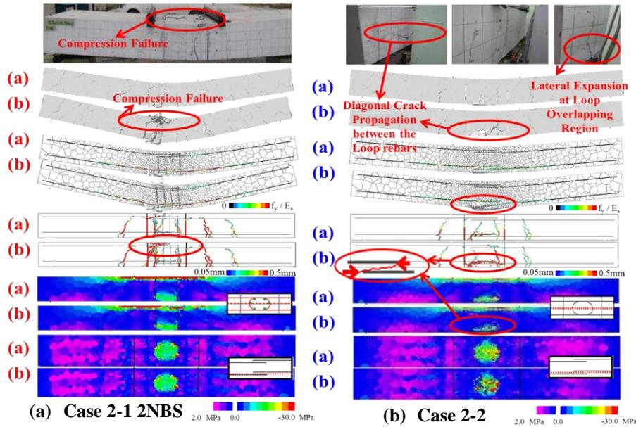
Fig. 10 Experiment photos, deformed shape, cracks pattern and stress distribution of Case 2
