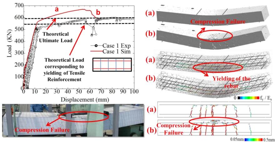
Fig. 8 Experimental and numerical simulation results of ordinary RC beam
