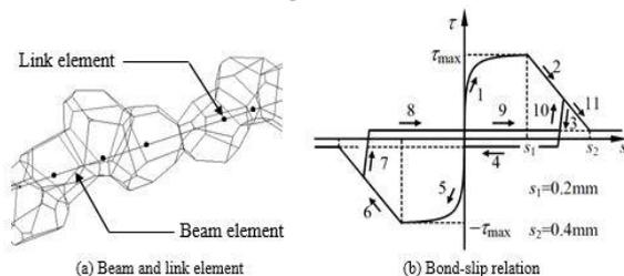
Fig. 3 Reinforcing bar and bond interface models (Yamamoto et al., 2014)
