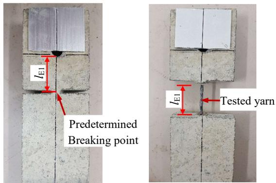
a) Before pull-out test      b) After pull-out test
