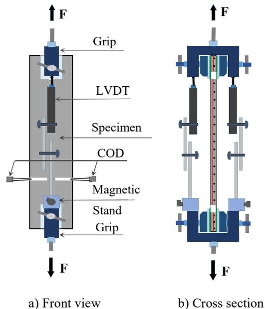
Fig.5 Sketch of Setup for pull-out test
