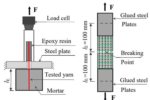
a) Test setup by Banholzer b) Test setup by Butler
