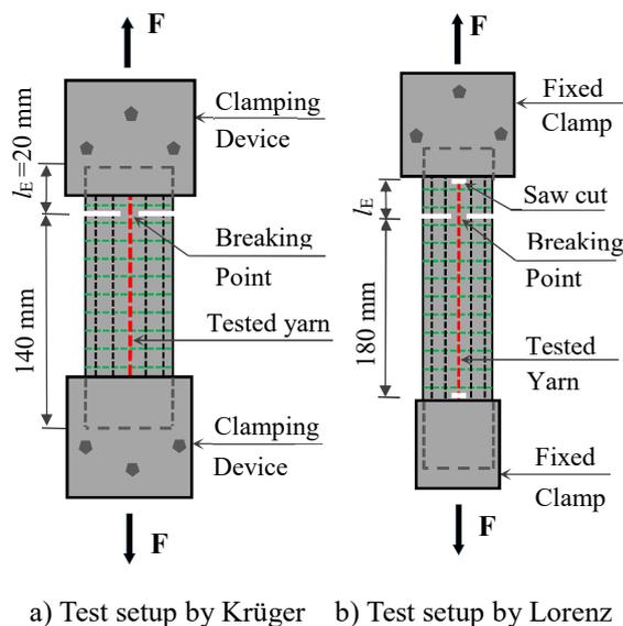
Fig.2 Setups of pull-out test proposed by Krüger [5], and Lorenz [6]
