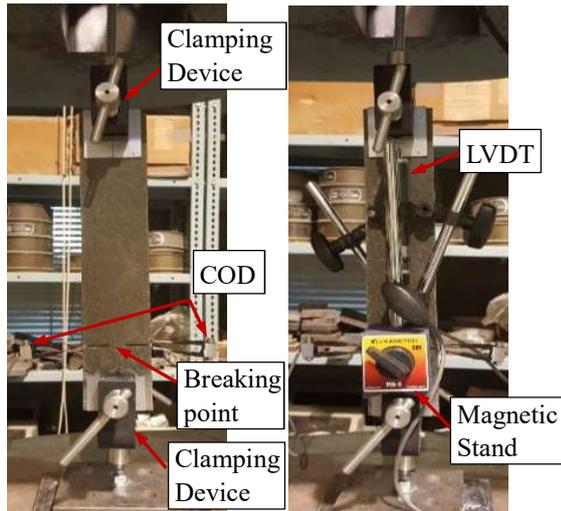
Fig.6 Setup of pull-out test
