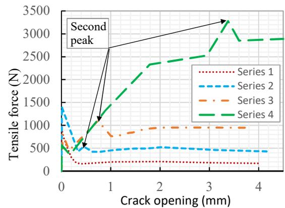
Fig.9 Tensile force – crack opening relationship of four series
