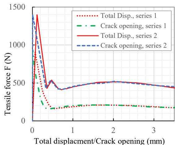
Fig.10 Correlation between total displacement and crack opening of series 1 and series 2
