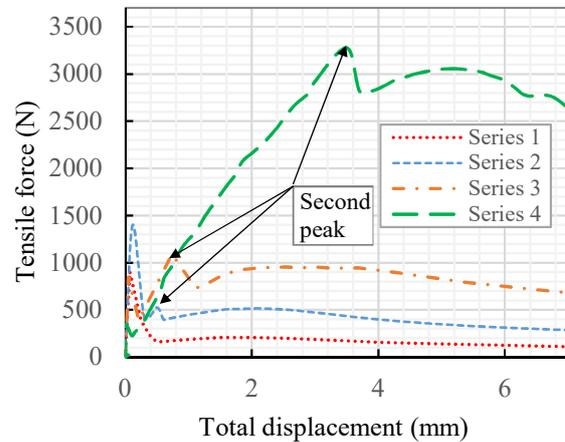
Fig.8 Tensile force – total displacement relationship of four series
