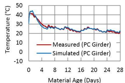
Fig. 6(c) Simulation of concrete temperature upon PC girder
