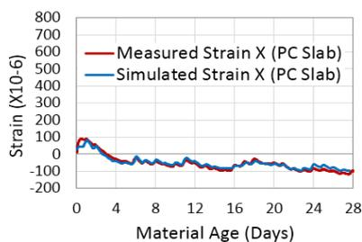
Fig. 7(a) Simulation of longitudinal (X) strain in concrete upon PC slab
