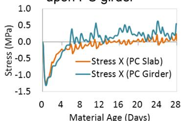
Fig. 9(a) Simulation of longitudinal stress in concrete
