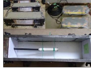
Fig. 3(a) Autogenous shrinkage specimens
