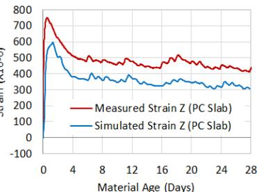
Fig. 7(c) Simulation of vertical (Z) strain in concrete upon PC slab
