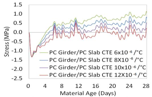
Fig. 11(a) Effect of CTE of PC girders/PC slabs on longitudinal stresses (upon PC girder)
