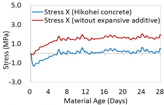
Fig. 10(a) Effect of expansive additive
