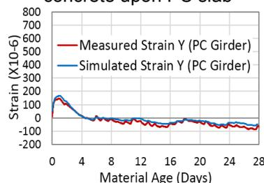
Fig. 8(b) Simulation of transverse (Y) strain in concrete upon PC girder
