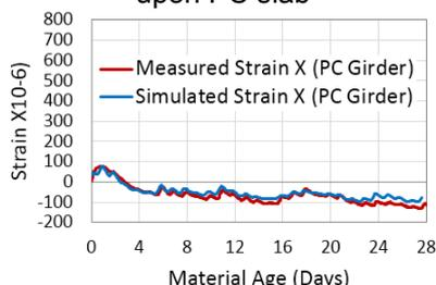
Fig. 8(a) Simulation of longitudinal (X) strain in concrete upon PC girder
