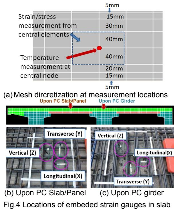
Fig.4 Locations of embedded strain gauges in slab
