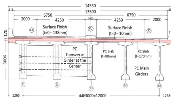
Fig. 1(a) Colored portions indicate the application of durable concrete for deck slab on Hikohei bridge
