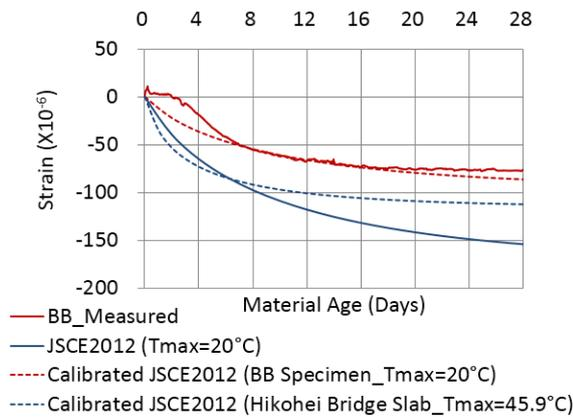
Fig. 3(b) Measured and calculated (modified JSCE2012 equation) autogenous shrinkage
