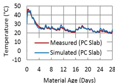
Fig. 6(b) Simulation of concrete temperature upon PC slab
