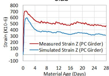
Fig. 8(c) Simulation of vertical (Z) strain in concrete upon PC girder
