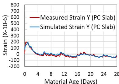
Fig. 7(b) Simulation of transverse (Y) strain in concrete upon PC slab
