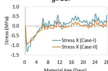
Fig. 9(c) Effect of C.R.F on concrete stress upon PC girder
