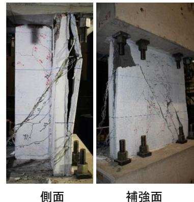
図-10 補強部剥離状況 (No. 2:W)
