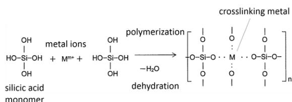
Fig. 1 Crosslinking and polycondensation [4]
