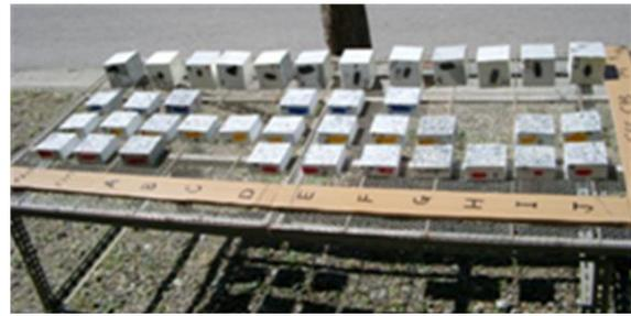
Photo 1 Specimens for Outdoor-Exposure Test.
