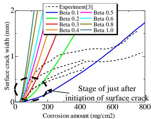
Fig. 10 Surface crack width propagation with various values of modification factor  $\beta$
