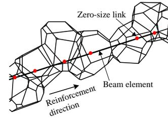
Fig. 3 Reinforcement arrangement
