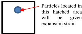
Fig. 5 UNIFORM corrosion model
