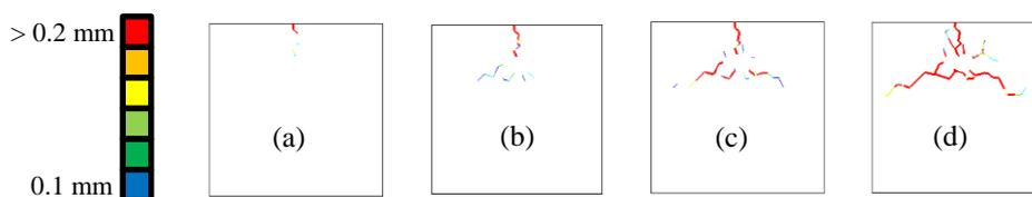
Fig. 15 Internal crack propagation
