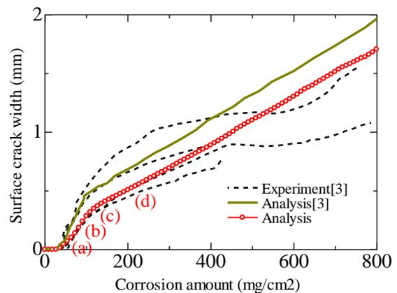
Fig. 13 Surface crack width propagation
