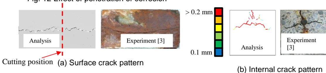
Fig. 14 Crack patterns compared with experiment
