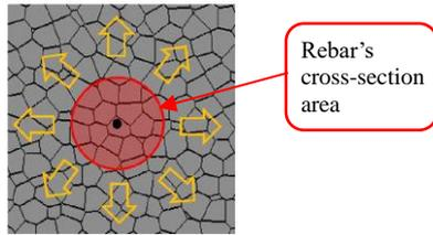
Fig. 4 Corrosion expansion model
