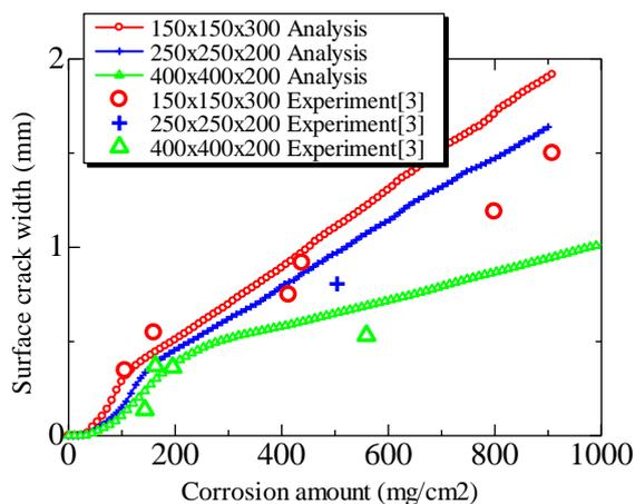
Fig. 20 Surface crack width propagation in cases of various sizes specimens
