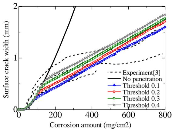
Fig. 12 Effect of penetration of corrosion
