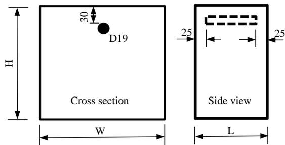
Fig. 18 Specimen set-up (various sizes)
