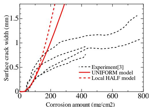
Fig. 11 Effect of local corrosion model
