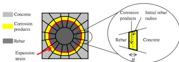
Fig. 1 Three-phase corrosion expansion model [3]
