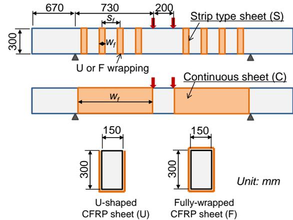
Fig. 2 Attaching layout of CFRP sheets
