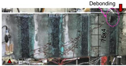
Fig. 11 Crack pattern at failure (B0-1.1SF)
