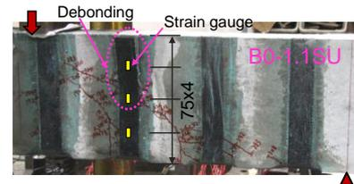
Fig. 8 Crack pattern at failure (B0-1.1SU)
