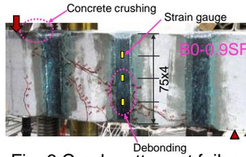
Fig. 6 Crack pattern at failure (B0-0.9SF)
