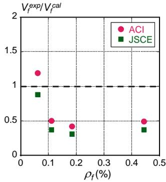
Fig. 13 Evaluation of equations in ACI and JSCE guidelines
