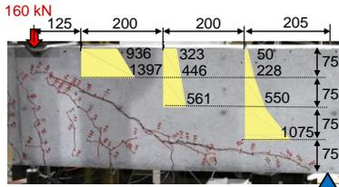
Fig. 5 Distribution of compressive strain (B0)
