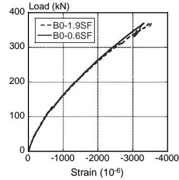
Fig. 13 Strain in concrete at midspan
