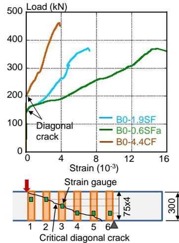
Fig. 4 Development of strain gauge 3
