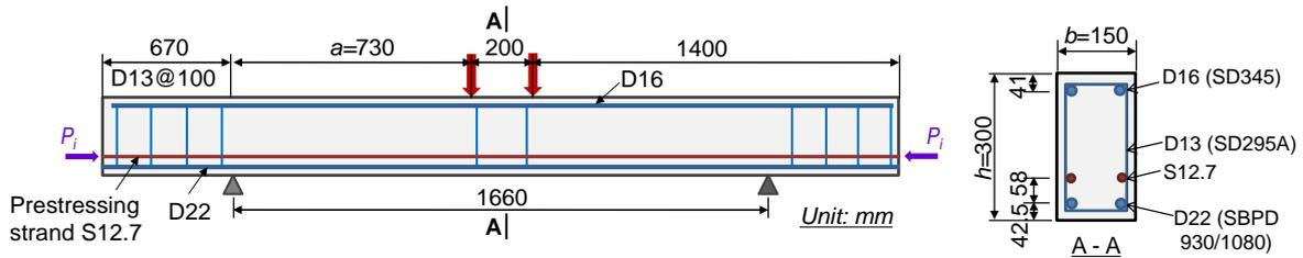
Fig. 1 Details of pretensioned PC beams
