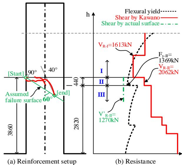
Fig. 9 Shear Resistance based on Actual Failure Surface
