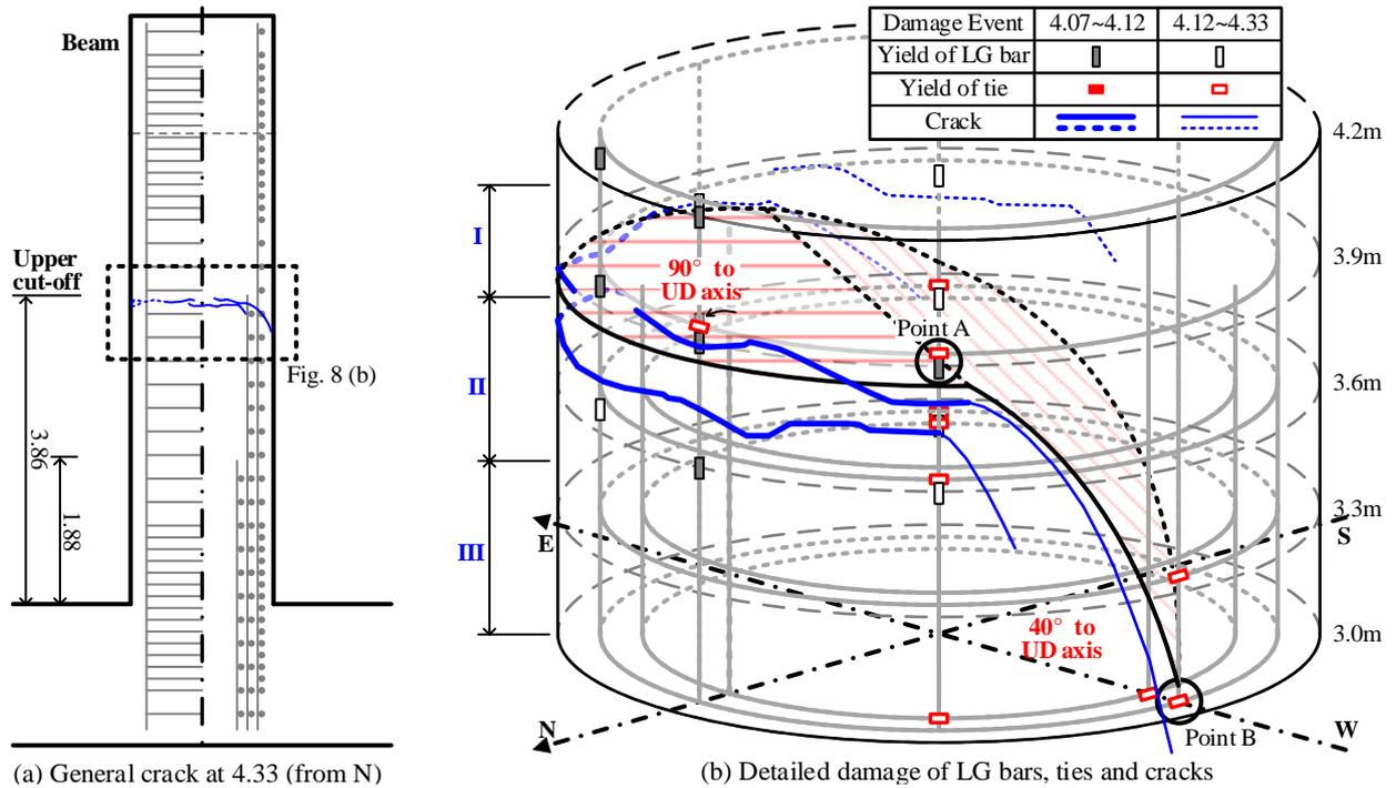
Fig. 8 Development of damage event (4.07–4.33 sec, at when shear crack occurred firstly)
