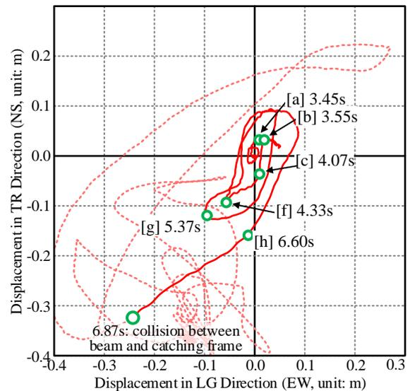
Fig. 4 Response Displacement History on Column Top
