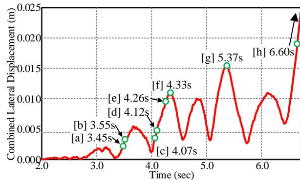
Fig. 5 Response History of Combined Lateral Displacement at Top of Column
