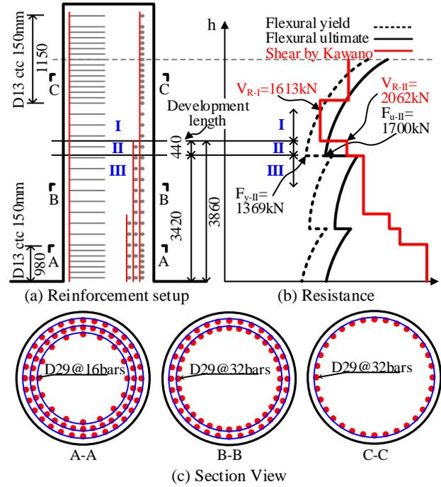
Fig. 2 Experimental Setup and Resistance Distribution
