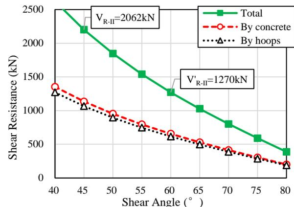
Fig. 10 Influence by Shear Angle on Shear Resistance
