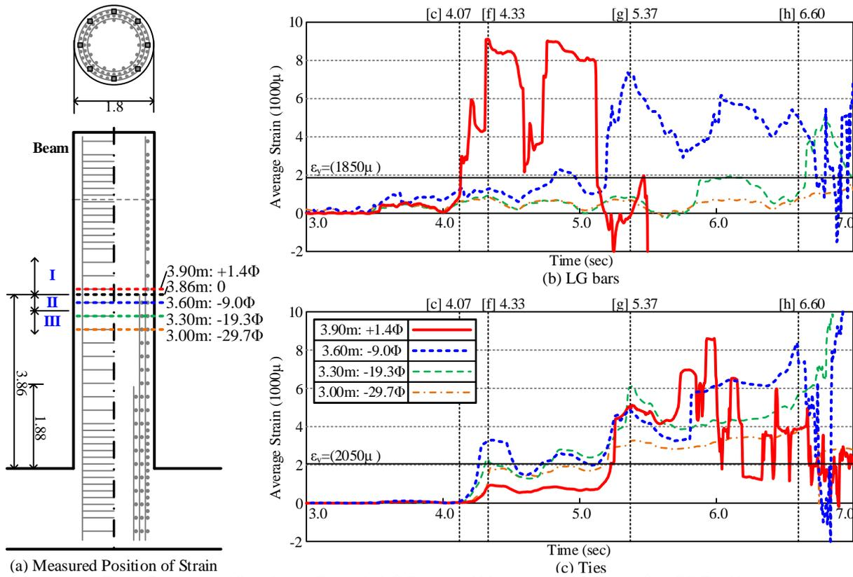
Fig. 7 Response Histories of Strain in LG Bars and Hoops around Upper Cut-Off Position
