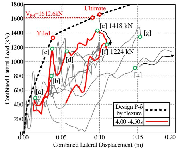
Fig. 6 Response Load-Displacement History on Top of Column
