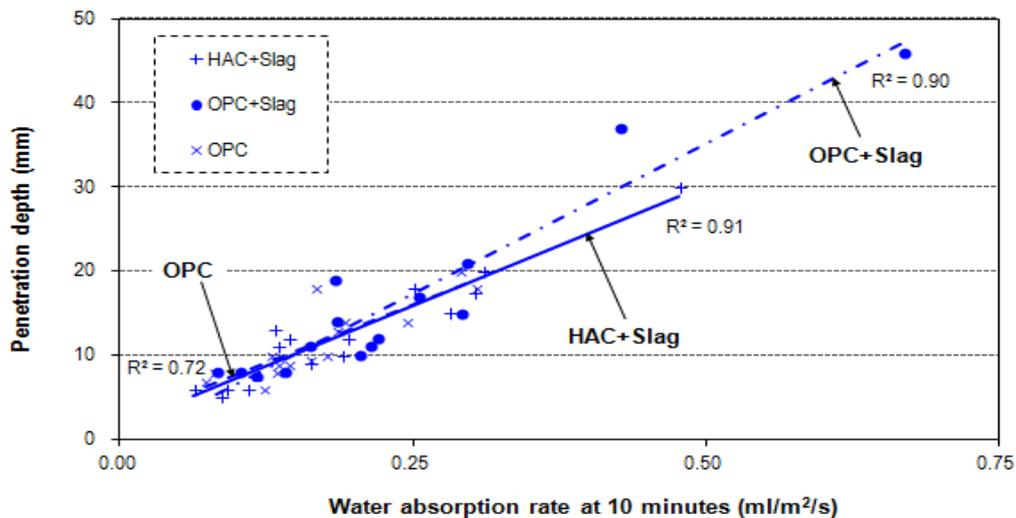
Fig. 9 Relationship between water absorption rate at 10 minutes and water penetration depth.
