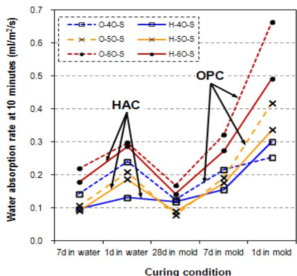
Fig. 8 Water absorption rate at 10 minutes of slag concretes with OPC and HAC.
