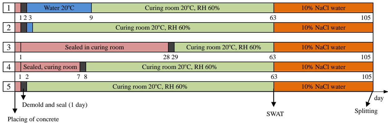
Fig. 1 Curing conditions and experimental process.
