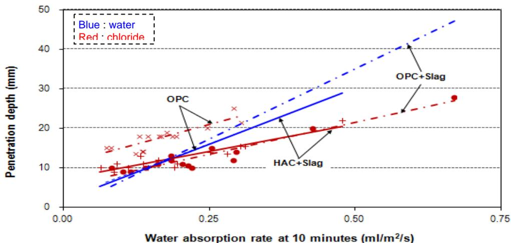
Fig. 10 Comparison between OPC, OPC slag, and HAC slag concretes.
