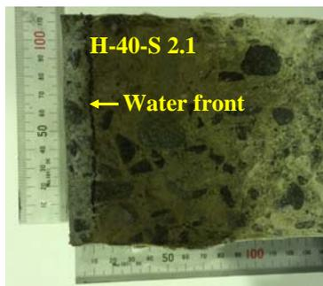
Fig. 5 Water front detected by naked eyes (black line).
