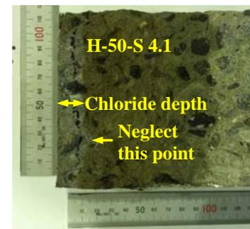
Fig. 7 Chloride front detected by  $\text{AgNO}_3$ .
