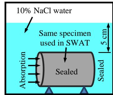
Fig. 4 Specimen was immersed in 10% NaCl water.
