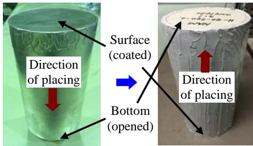
Fig. 2 Specimen was wrapped by alumina tape (left) and then coated by epoxy resin (right).
