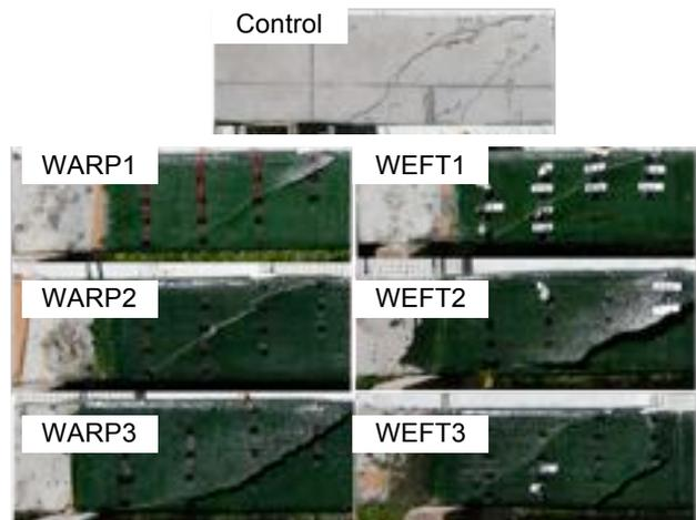
Fig. 4 Failure modes before removing fiber sheets
