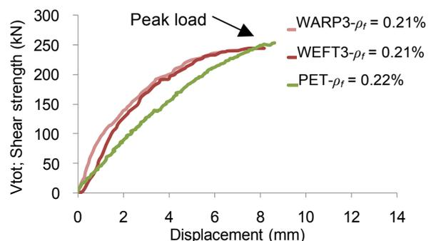
Fig. 13 Comparison between RC beams jacketed by flax FRP and PET FRP sheets
