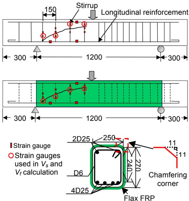
Fig. 3 Characteristics of beam specimens, test setup and location of strain gauges
