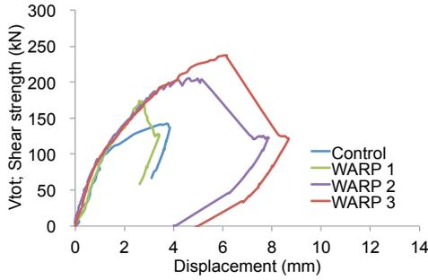
Fig. 6 Relation between shear force and vertical displacement of WARP specimens
