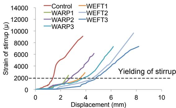
Fig. 11 Strain increments of stirrups
