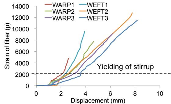
Fig. 12 Strain distributions of flax-FRP sheets
