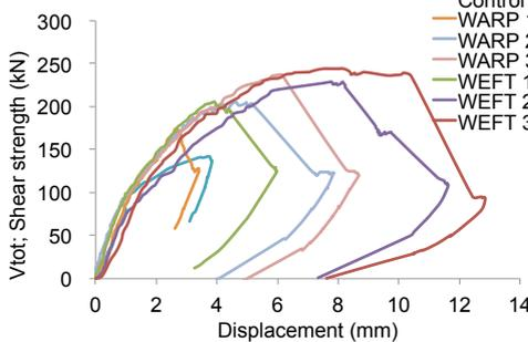
Fig. 8 Relation between shear force and vertical displacement of RC beams
