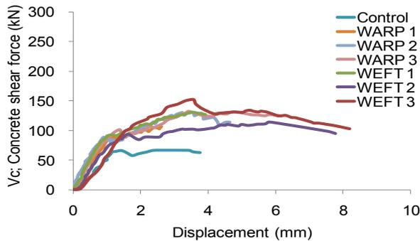
Fig. 10 Relationship between concrete shear force and vertical displacement
