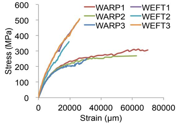
Fig. 2 Stress-strain curve of coupon specimens
