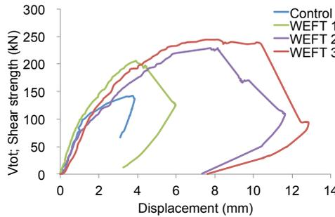
Fig. 7 Relation between shear force and vertical displacement of WEFT specimens
