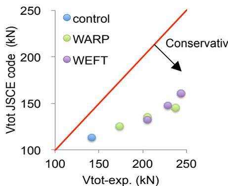
Fig. 14 Comparison between shear strength from experiment and JSCE code
