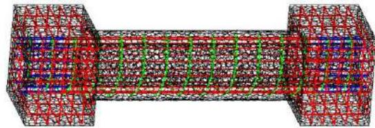
Fig.5 Reinforcement Arrangement
