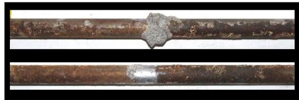
Photo 6 A View of Steel Corrosion After 15cycles
