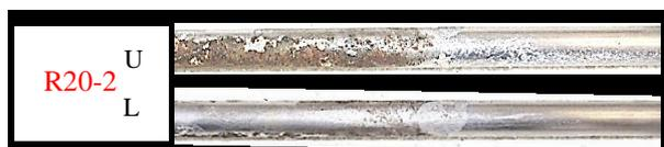
Photo 5 A View of Steel Corrosion After 20cycles
