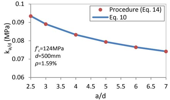
Fig.5 Influence of  $a/d$  on shear strength
