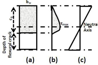
Fig.4 Shear stress distribution: (a) cross-section, (b) shear stress distribution, and (c) longitudinal strain distribution (where,  $\tau_{max}$  is the maximum shear stress in effective shear depth)
