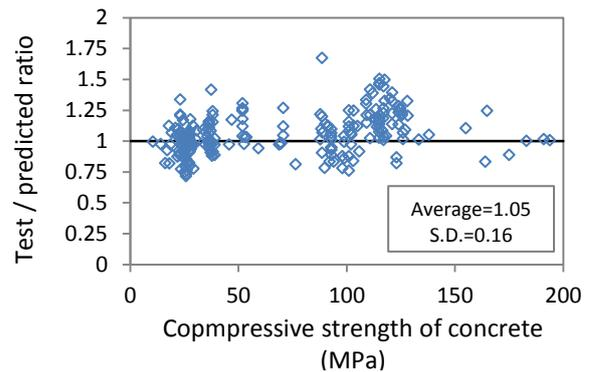
Fig.6 Comparison of experimental results with proposed equation: influence of compressive strength of concrete.
