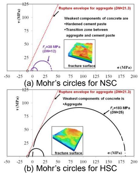
Fig.1 Mohr's circles for rock and concrete ( $f'_c$  is compressive strength of concrete) [10]
