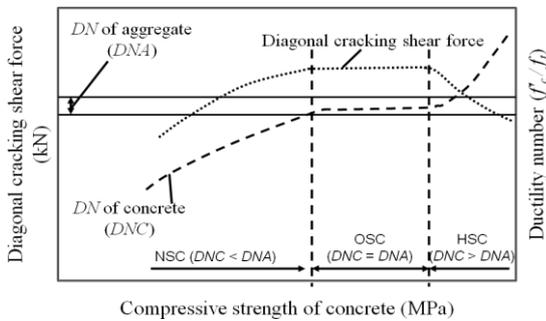
Fig.2 Effect of compressive strength of concrete on  $DN$  and diagonal cracking shear force of RC members (NSC: Normal strength concrete, OSC: Optimal strength concrete, HSC: High-strength concrete)
