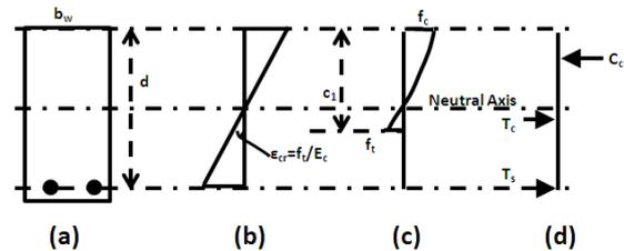
Fig.3 Strain compatibility and force equilibrium at section: (a) cross-section; (b) strain distribution, (c) stress distribution, (d) force distribution (where,  $\epsilon_{cr}$  is cracking strain in concrete,  $C_c$  is compressive force due to concrete,  $T_c$  is tensile force due to concrete, and  $T_s$  is tensile force due to main steel)
