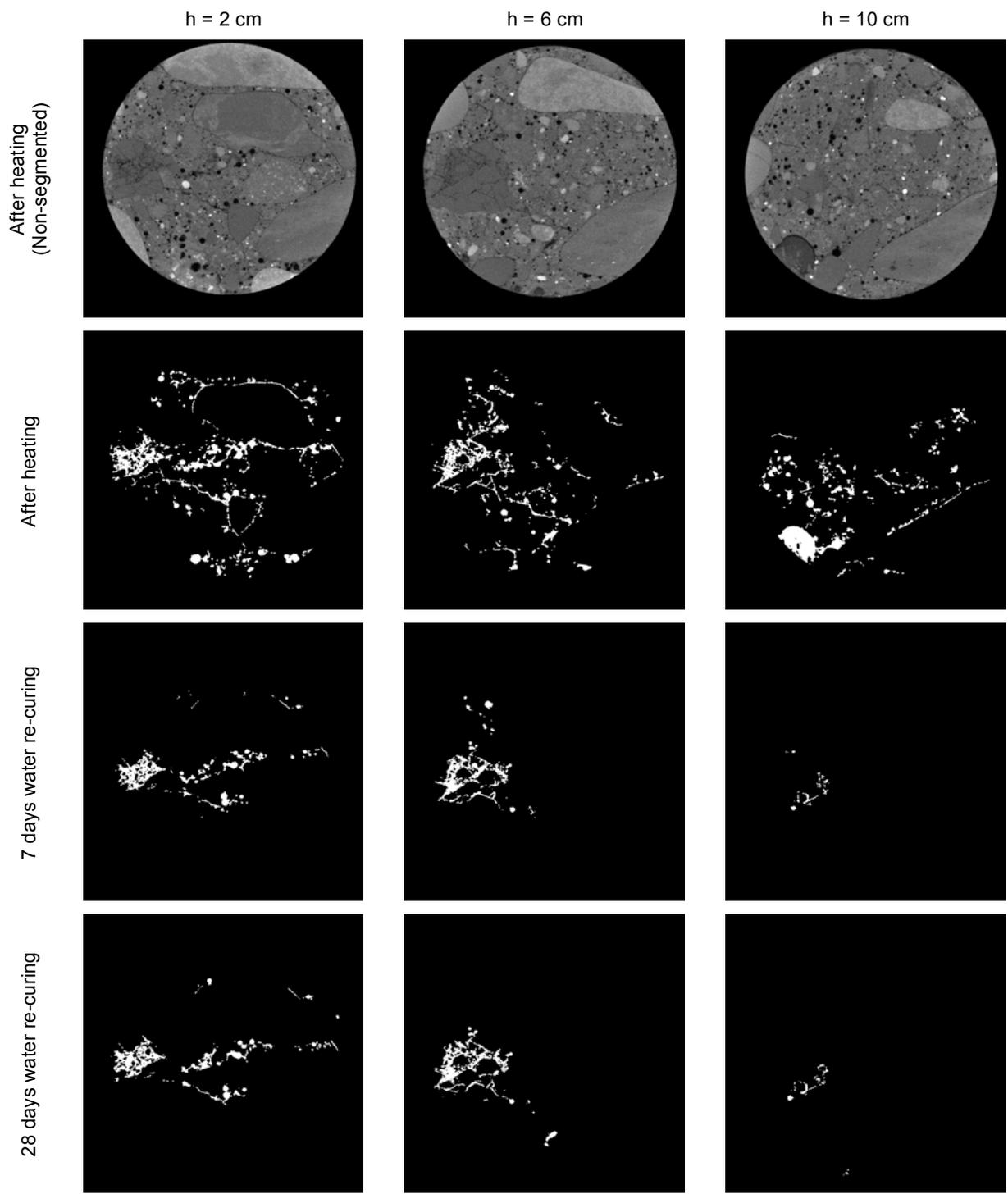
Fig. 5 Comparison of percolated void space after heating and re-curing at various heights
