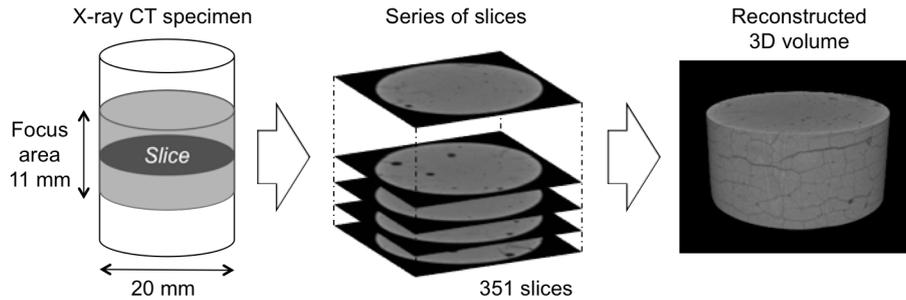
Fig. 2 Details of the X-ray CT specimen and 3D digital image reconstruction
