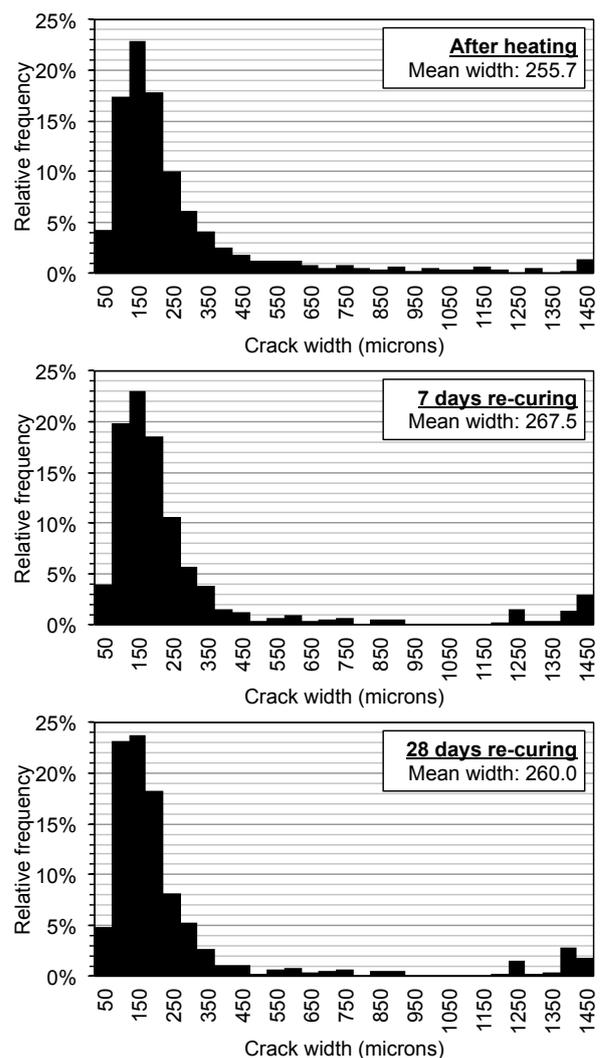
Fig. 7 Crack width distributions
