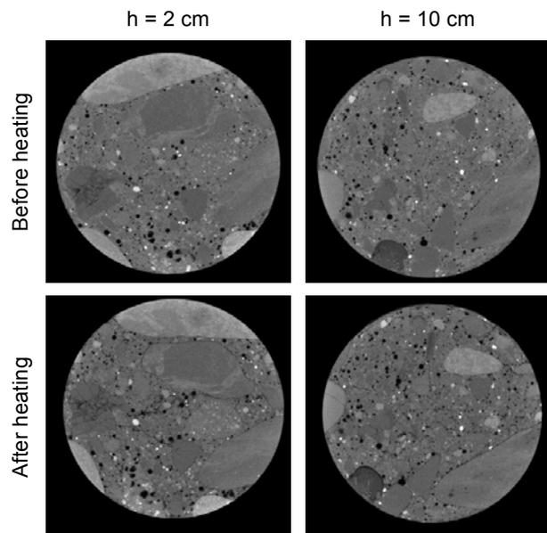
Fig. 3 Cross sections from before and after heating
