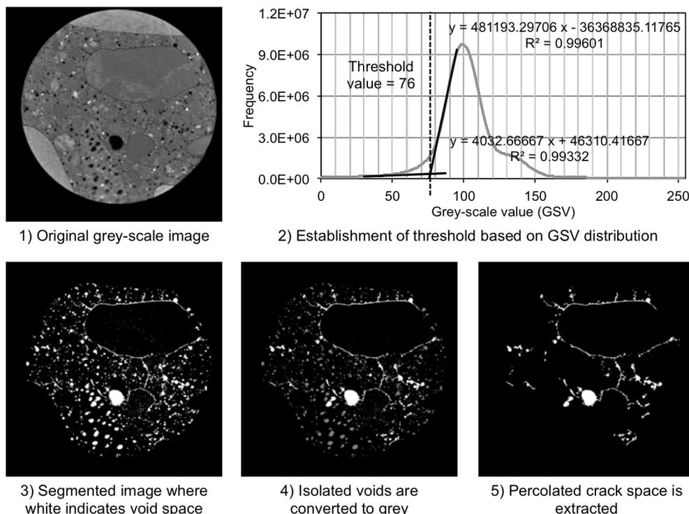
Fig. 4 Method of segmentation for extracting percolated crack space
