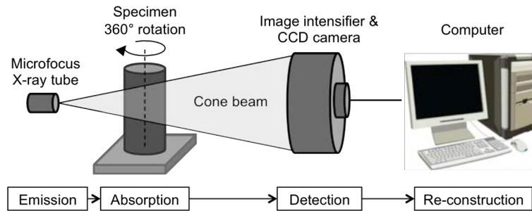
Fig. 1 Set-up for the X-ray CT image acquisition
