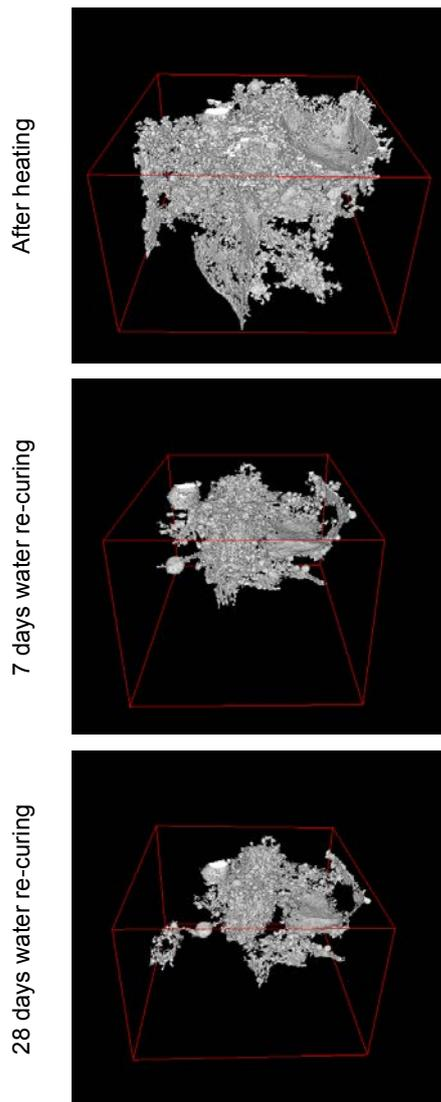
Fig. 6 Three-dimensional crack networks
