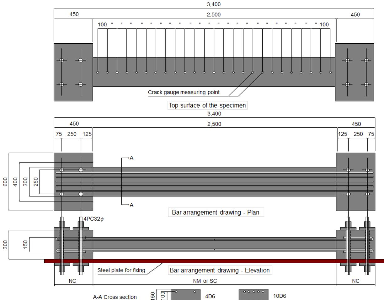
Fig.3 Specimens of restrained drying shrinkage test
