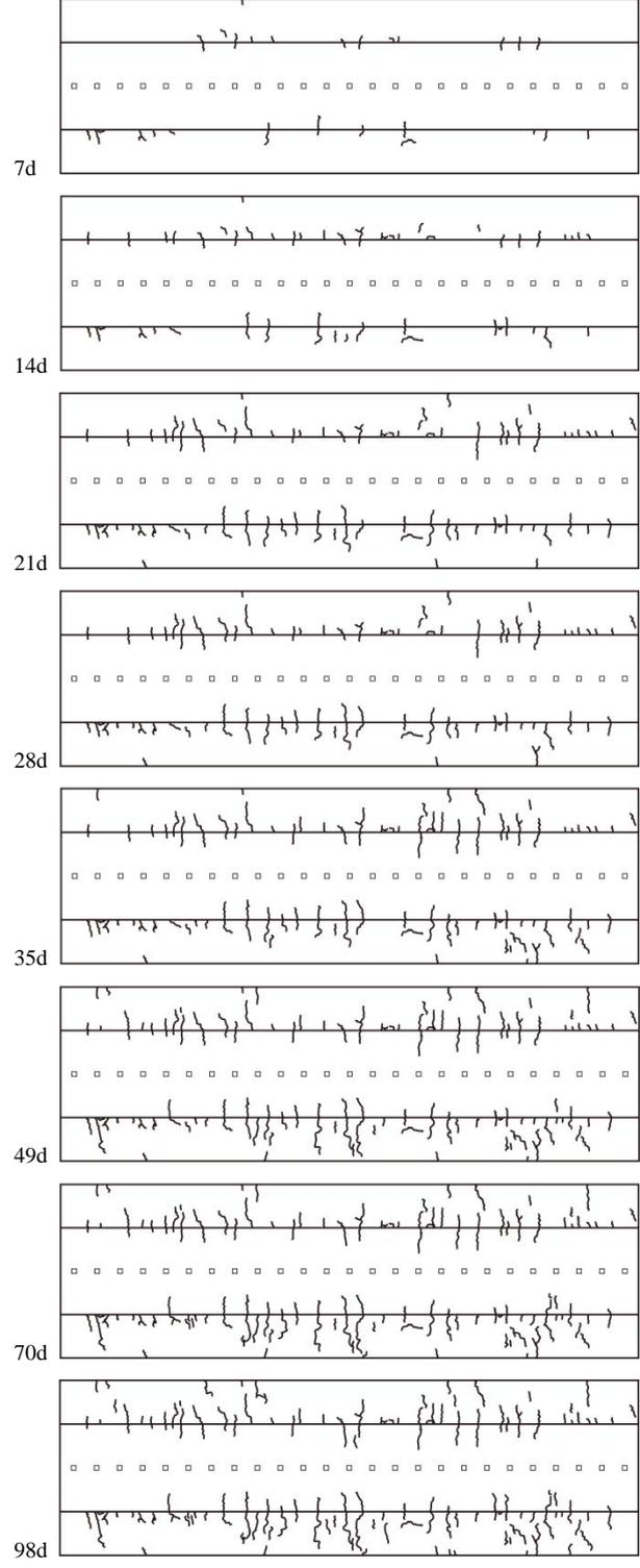
Fig.10 Drying shrinkage and crack patterns of specimen NM10
