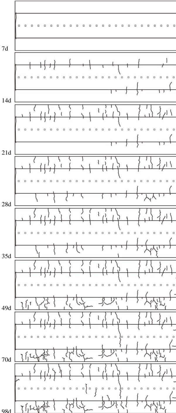
Fig.8 Drying shrinkage and crack patterns of specimen NM4
