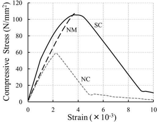
Fig.2 Relationship between compressive stress and strain of cementitious composites
