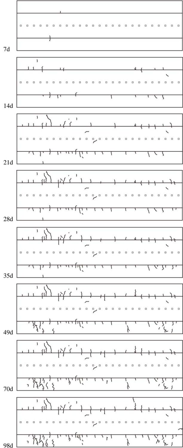
Fig.9 Drying shrinkage and crack patterns of specimen SC4
