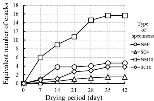
Fig.12 Relationship between equivalent number of cracks of specimens and drying period
