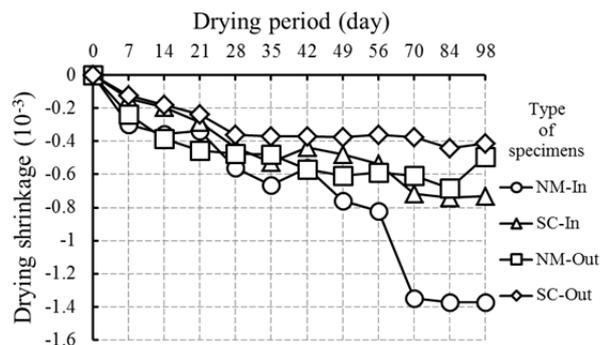
Fig.7 Relationship between drying shrinkage of free shrinkage specimens and drying period
