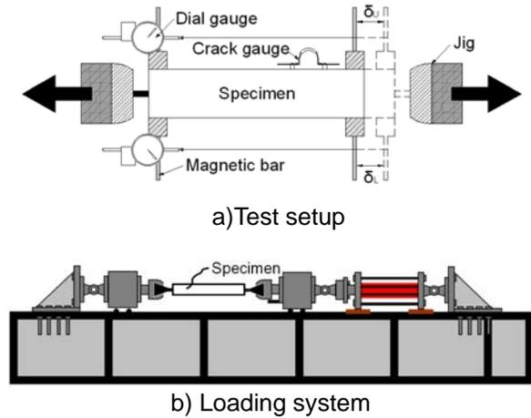
Fig. 2 Test setup of rebar lap splice specimens
