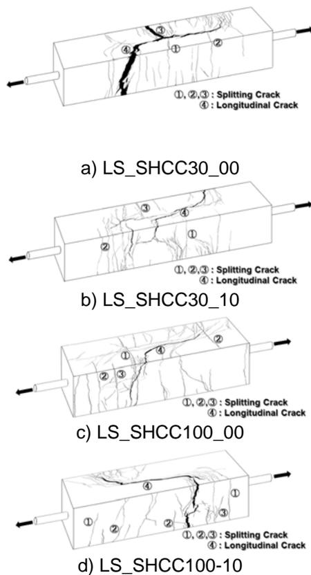
Fig. 8 Typical crack patterns of lap splice specimens
