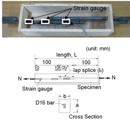
Fig. 1 Configuration and dimension of rebar lap splice specimen
