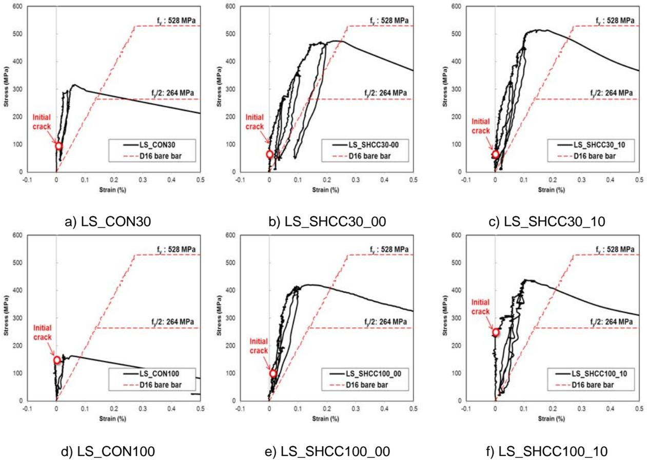
Fig. 6 Tensile response of lap splice specimens
