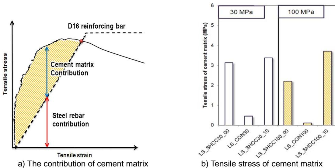
Fig. 7 Tensile stress carried by cement matrix in the lap splice specimen
