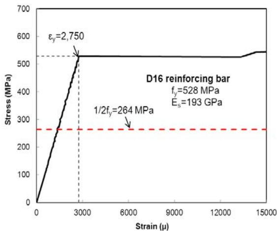
Fig. 3 Stress-strain relationship of reinforcing bar
