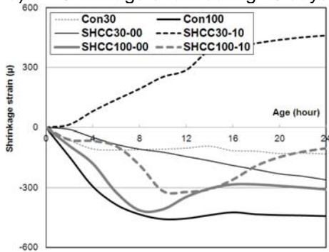
b) Shrinkage strain during 24 hours
