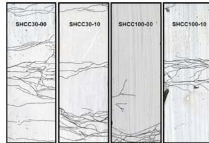
b) Typical crack patterns of SHCCs
