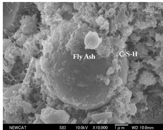
Photo 3 SEM Photo of ②[3h Steam(80°C) Cured] Non-Burnt Brick Specimen (FA:India) (Crack:None) (×10000)
