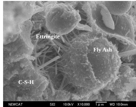
Photo 2 SEM Photo of ①[3h Steam(80°C) Cured] Non-Burnt Brick Specimen (FA:Japan) (×10000)
