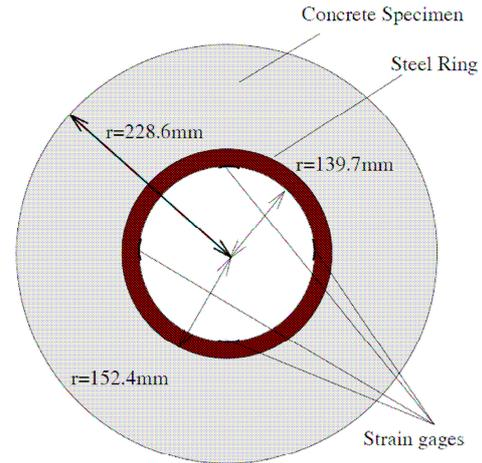
Fig.4 Detail of Ring Specimen
