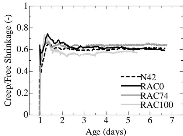
Fig.10 Ratio of Creep to Free Shrinkage
