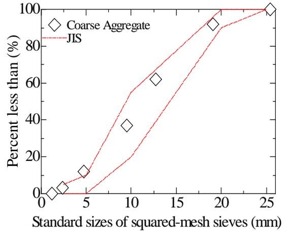
Fig.2 Size Distribution of Coarse Aggregate
