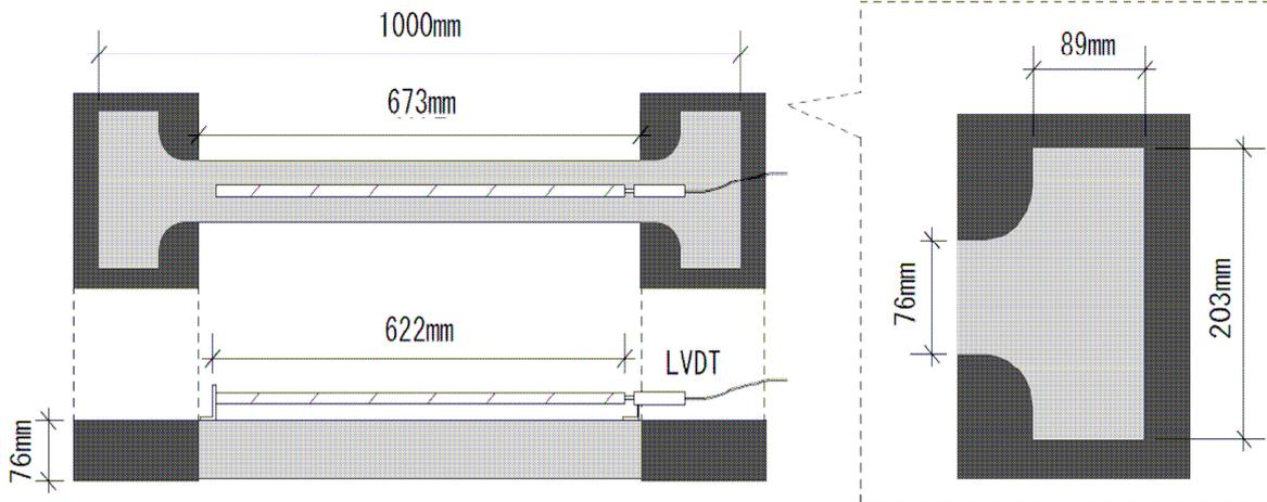
Fig.3 Uniaxial Tensile Loading Device
