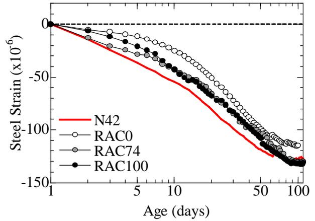
Fig.11 Steel Strain with Ages
