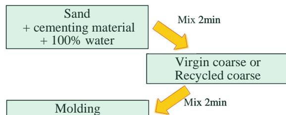
Fig.1 Mixing Procedures of TSM and SM absorbed into recycled coarse aggregate at first mixing. Therefore, this study focus on the influence of initial moisture content of recycled coarse aggregate on the various components of tensile creep in RAC made with TSM or single mixing (SM).
