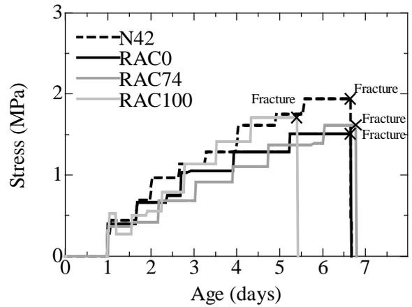
Fig.7 Stress Developing in Uniaxial Specimen
