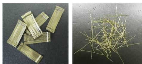
Fig. 4- Hooked and Twisted fibers
