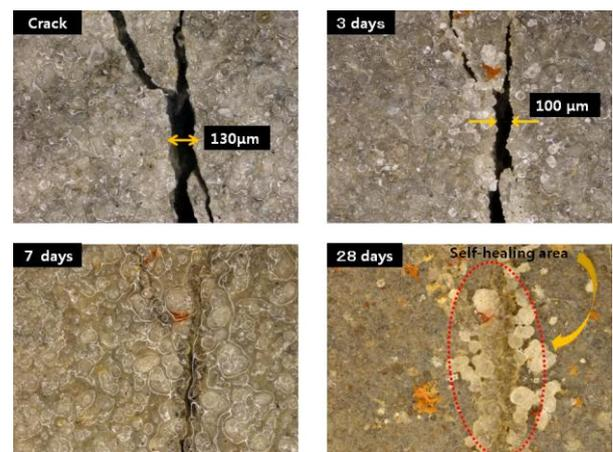
(b) Crack width ( $130 \mu\text{m}$ ,  $100 \mu\text{m}$ ) (B area)
