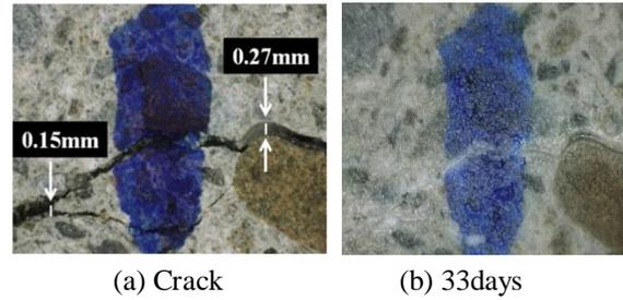
Fig. 2- Self healing behavior of Concrete (Ahn and Kishi [12])
