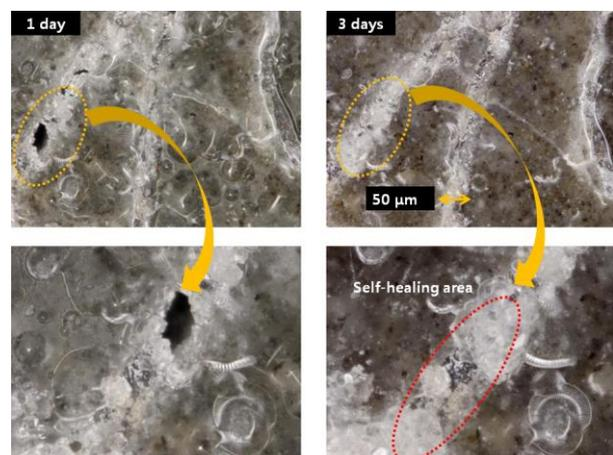
Fig. 9- Process of self-healing on Matrix A with twisted fiber 2% (Crack width  $50 \mu\text{m}$ )
