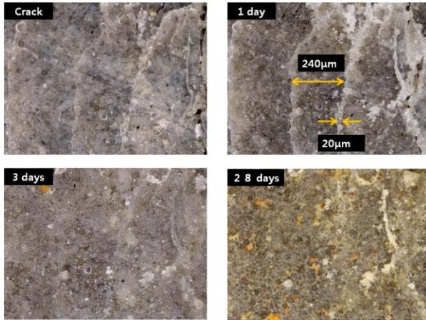
Fig. 10- Process of self-healing on Matrix B with twisted fiber 2% (Crack width 20  $\mu\text{m}$ )
