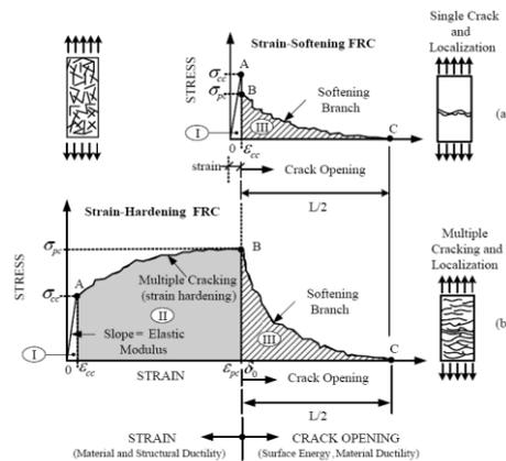
Fig. 1 – Typical tensile strain softening and hardening behavior of FRC, HPFRCC and UHP-FRC (Naaman and Reinhardt [1])
