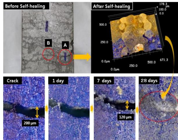
(a) Crack width ( $200 \mu\text{m}$ ) (A area)
