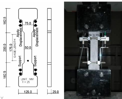
Fig. 5- The geometry of tensile test specimen and set-up
