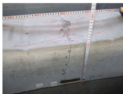
(a) S-1 (曲げ破壊)
