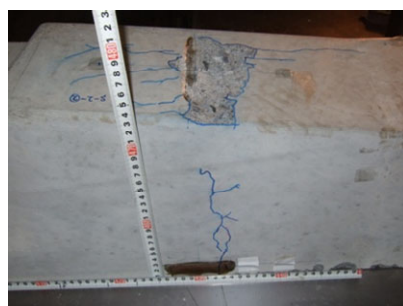
(c) S-3 (曲げ破壊)
