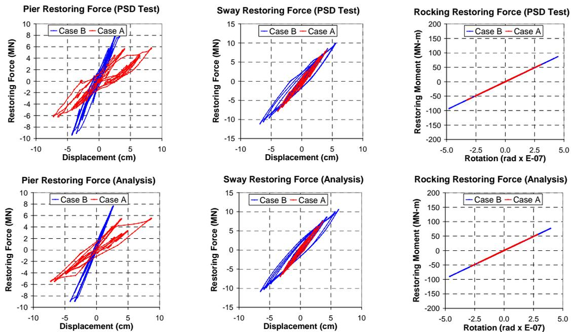
Fig. 9 Load-displacement hysteresis of Case A vs. Case B - PSD test (Upper) and Analysis (Lower)
