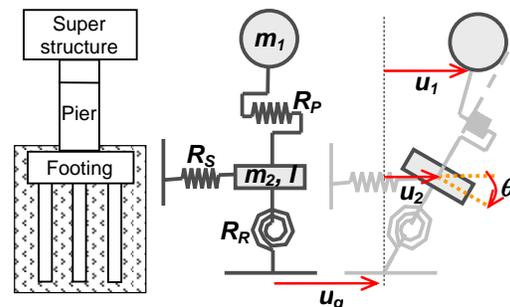
Fig. 1 The 3-DOF model used in PSD test
