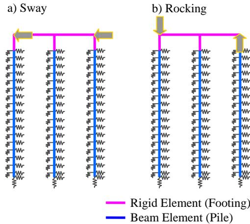
Fig. 3 Foundation model used the calculation of load-displacement relationship in soil springs
