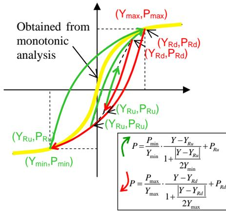
Fig. 4 HD-model used in sway spring
