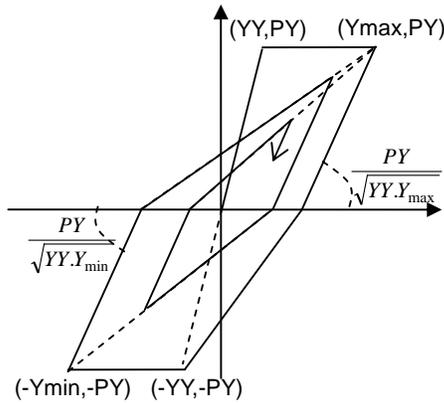
Fig. 7 Bi-linear model used in the analysis of pier
