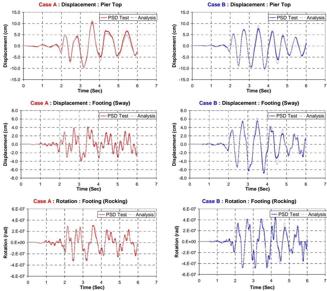
Fig. 8 Displacement results of Case A and Case B
