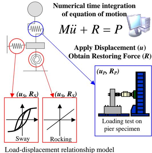
Fig. 6 Experimental set up of PSD test
