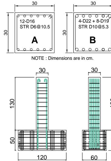
Fig. 5 Scaled down specimens
