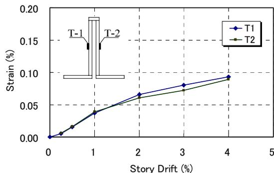
Figure 13 Strain of the U-shaped steel box drift increased. This improves that the U-shaped steel box has worked well to transfer the beam shear force to the bracket.
