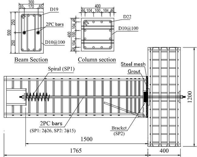
Figure 1 Reinforcement details of specimens SP1, SP2
