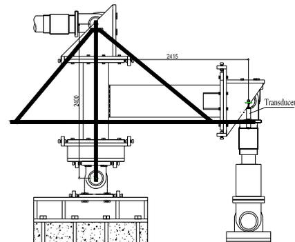
Figure 5 Measurement system of story drift
