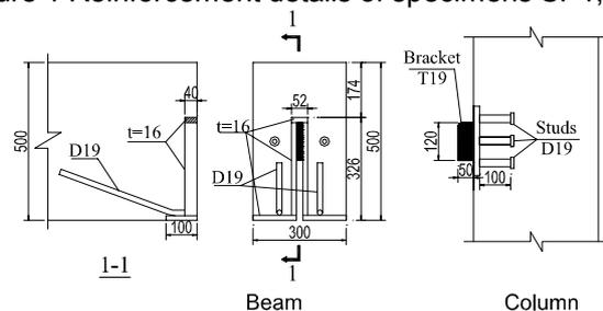
Figure 2 Details of the shear bracket, SP2
