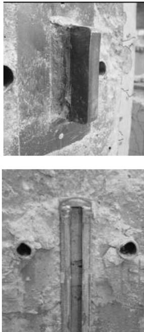
Figure 7 Shear bracket and inverted U-shaped steel box after testing
