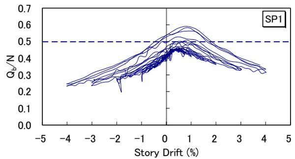
Figure 11 Variation of beam shear force/PC force ratio
