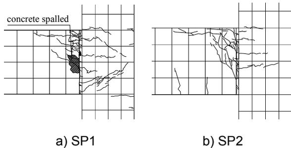
Figure 6 Crack pattern of specimens after 4% drift
