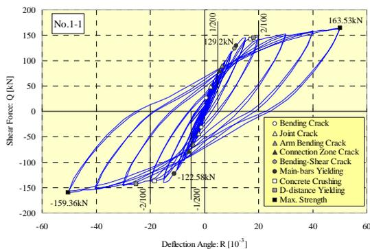
Fig.8 Load response of beam No.1-1
