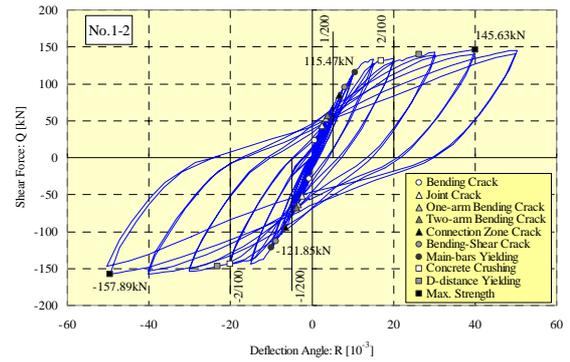
Fig.10 Load response of beam No.1-2
