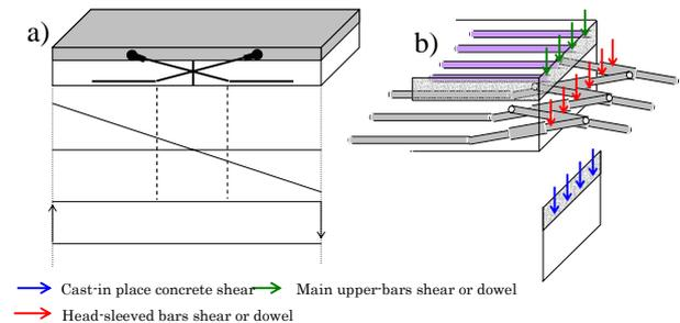
Fig.7 Moment and shear distribution (a), and assumed forces at connection of crossed-bars beam No.3-2 (b)
