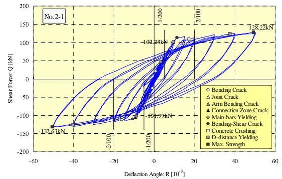
Fig.12 Load response of beam No.2-1
