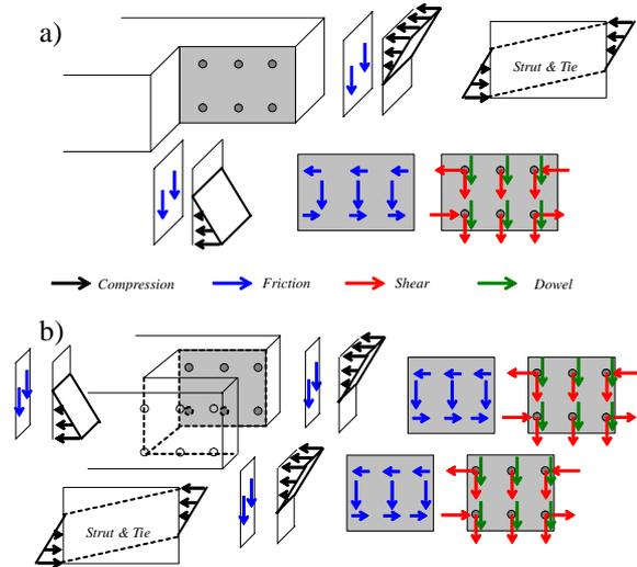
Fig.5 Assumed forces at connection of a one-arm beam No.1-1 (a) and a two-arm beam No.1-2 (b)
