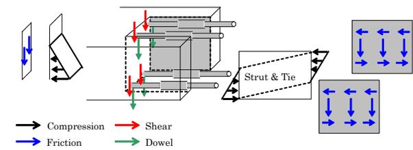
Fig.6 Assumed forces at connection of sleeved beam No.2-1
