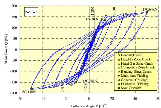
Fig.14 Load response of beam No.3-2
