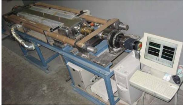
Fig.1 Temperature-stress testing machine (TSTM)
