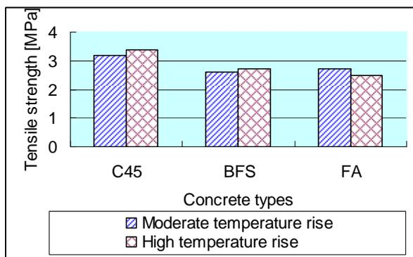
Fig.3 Tensile strength of concrete
