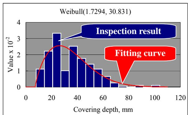
Fig.4 Distribution fitting of the inspection result
