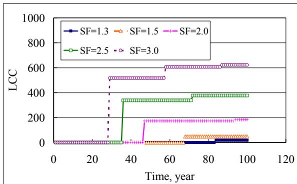
Fig.7 Life cycle cost based on using safety factor
