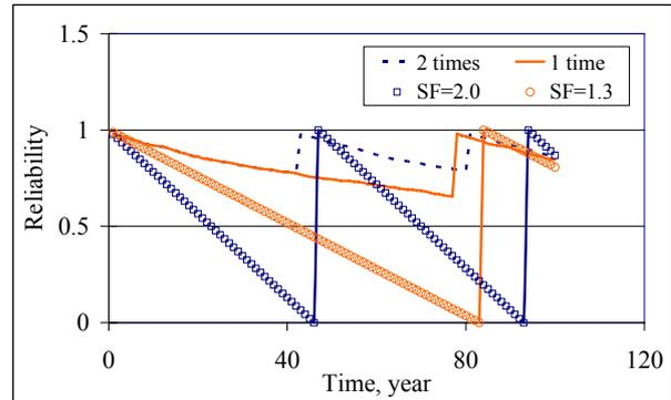
Fig.9 Reliability of structure along service life
