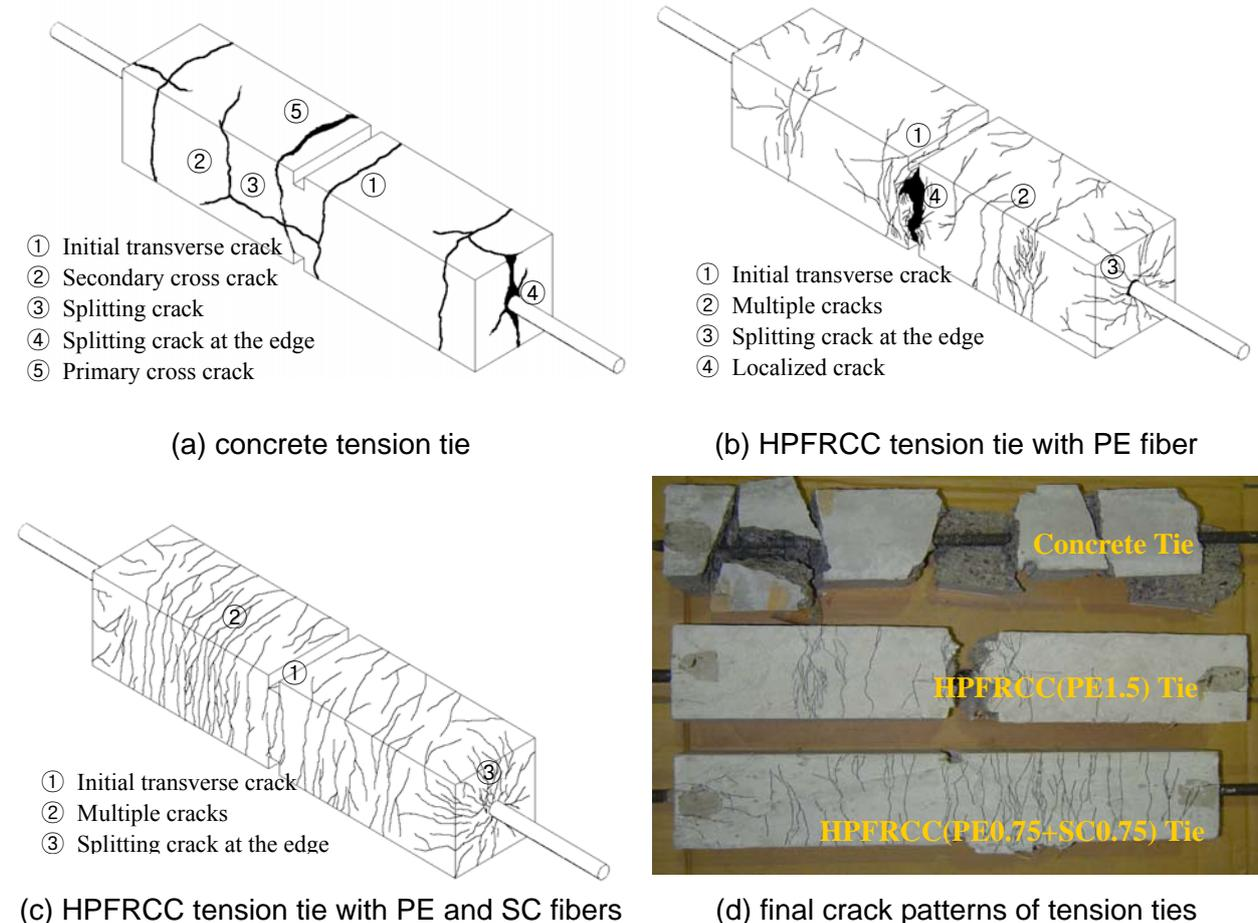
Figure 4 Cracking procedure and final failure patterns of tension ties
