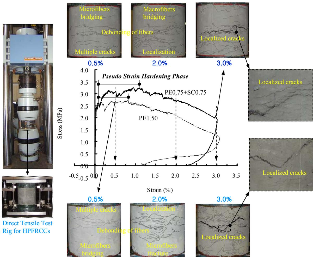
Figure 1 Typical tensile response and fracture process of HPFRCCs
