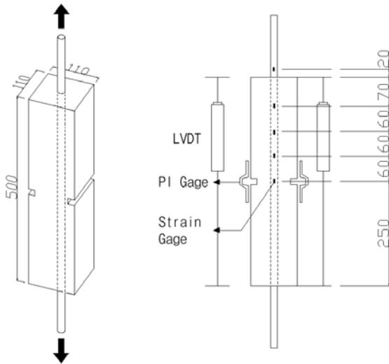
Figure 2 Tension tie details (unit :mm)
