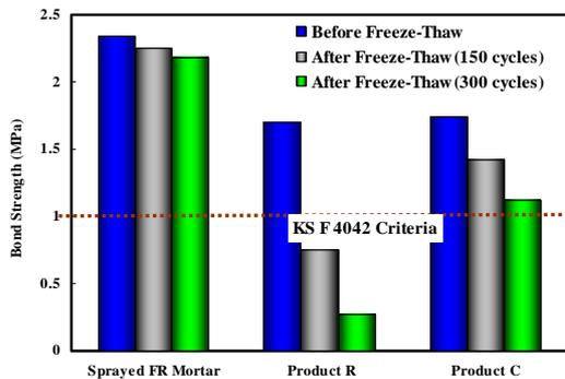
Fig. 9 Comparison of Bond Strength before and
