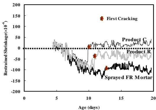
Fig. 6 Strain due to confining shrinkage
