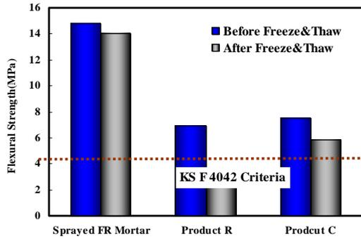
Fig. 8 Change of the flexural strength before and after freezing-thawing test
