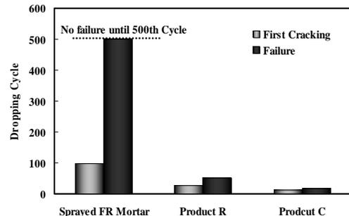
Fig. 4 Impact strength according to the type of repair material
