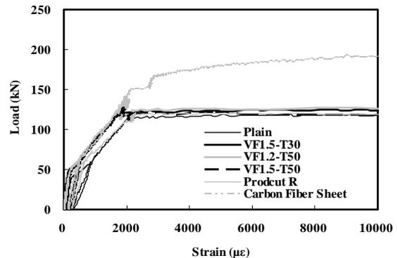
Fig. 11 Relationships of Load versus strain of rebar
