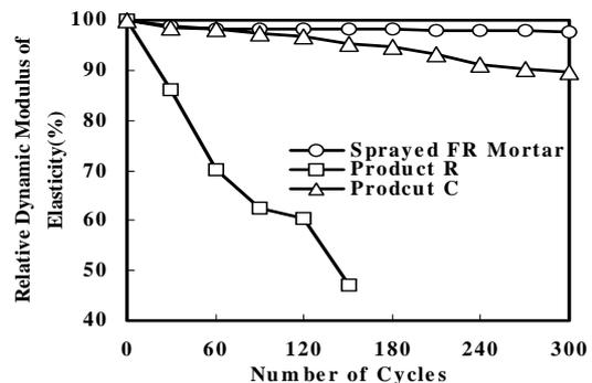
Fig. 7 Results of relative dynamic modulus of elasticity
