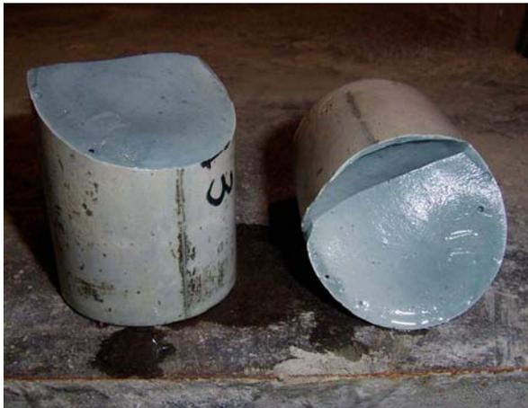
Photo 1 Cement paste broken by sodium
