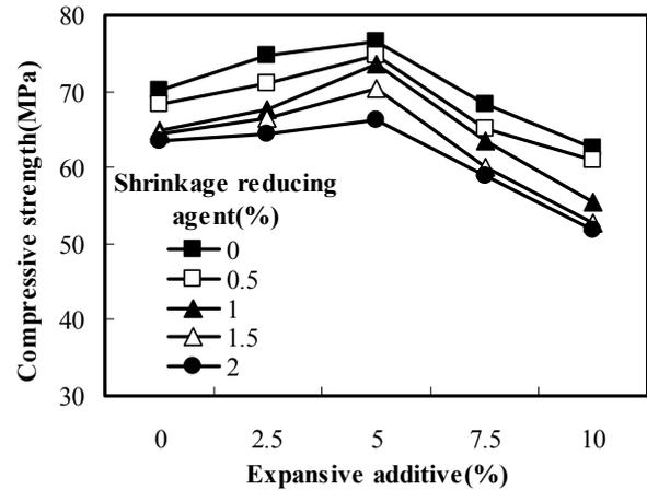
Fig. 3 Compressive strengths at 28 days
