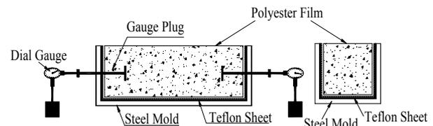
Fig. 1 Set up of autogenous shrinkage test device
