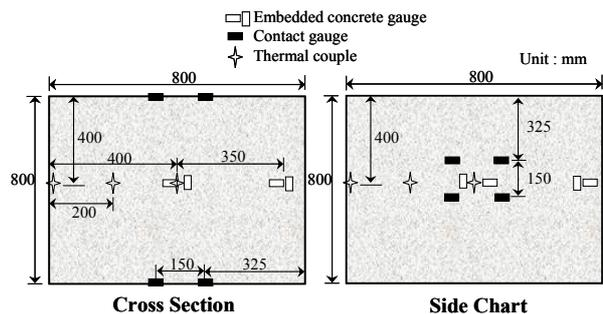
Fig. 2 Specimen for mock-up test
