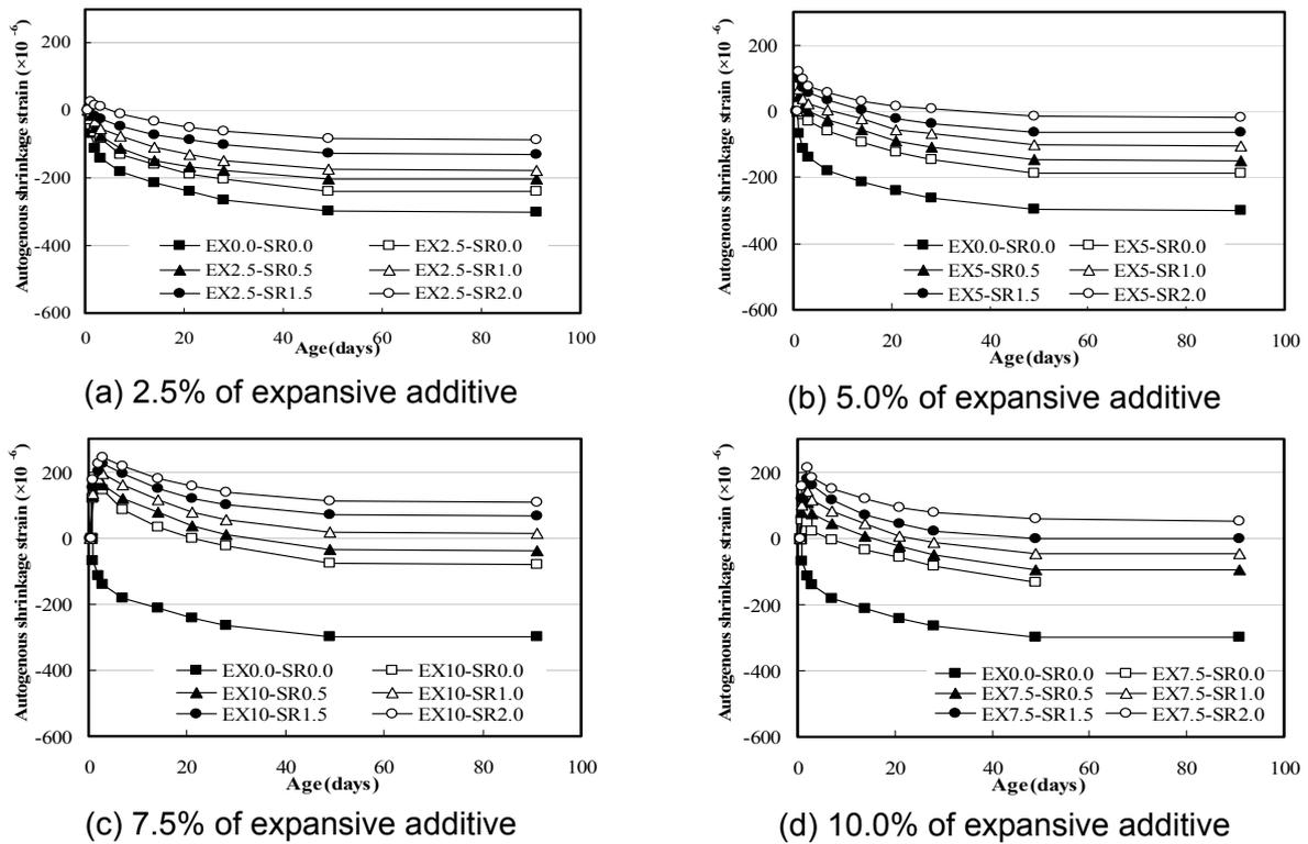
Fig. 6 Effect of expansive additives and shrinkage reducing agents on the autogenous shrinkage of high performance concrete
