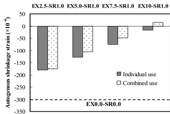
Fig. 7 Effect of expansive additives and shrinkage reducing agents on the autogenous shrinkage
