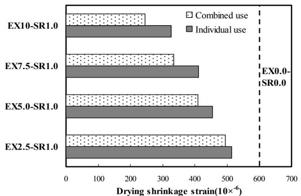
Fig. 5 Effect of expansive additive and shrinkage reducing agent on the drying shrinkage
