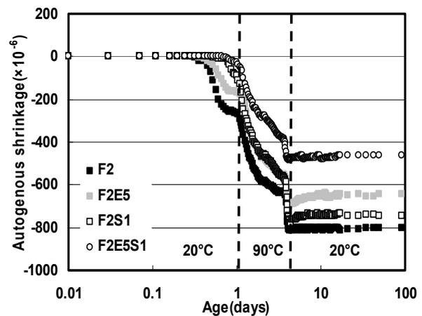
Fig. 4 Effect of the expansive additive and shrinkage reducing agent on the autogenous shrinkage
