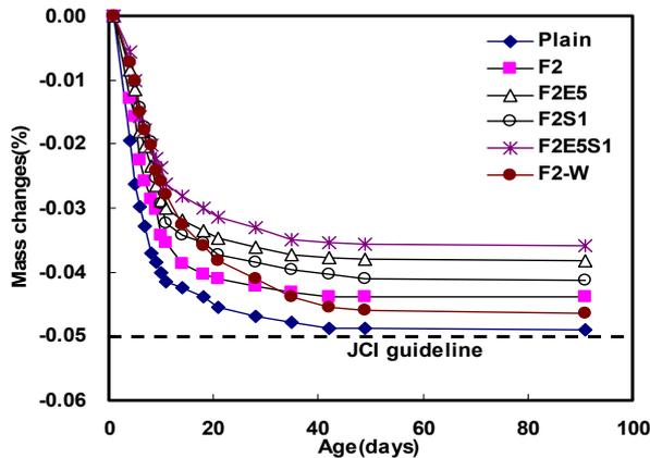
Fig. 6 Mass changes of the specimens during autogenous shrinkage tests
