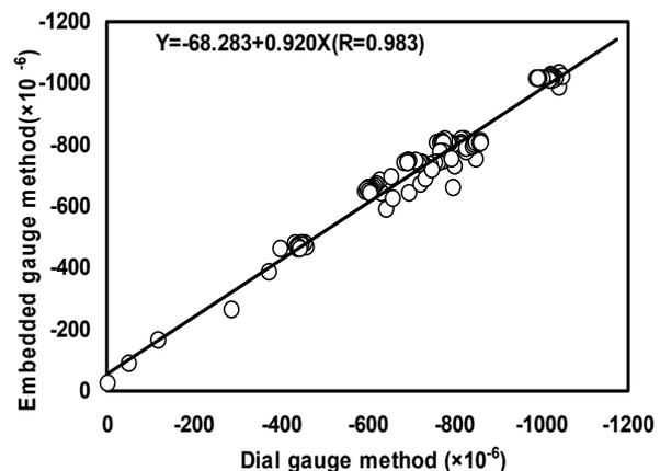
Fig. 5 Effect of the measurement method on the autogenous shrinkage
