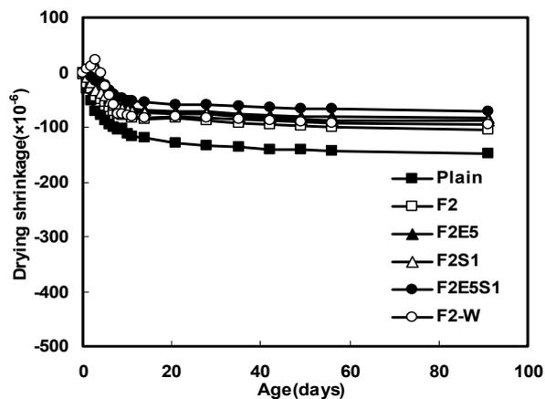
Fig. 7 Results of drying shrinkage test
