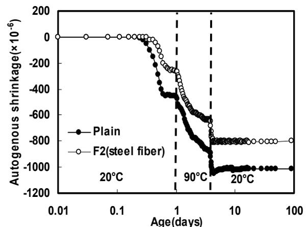
Fig. 2 Effect of the mixing of steel fibers on the autogenous shrinkage
