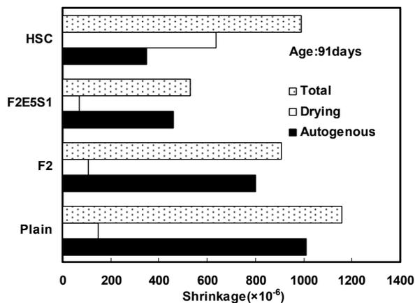
Fig. 10 Comparison of the shrinkage properties of ultra-high strength SFRC and HSC
