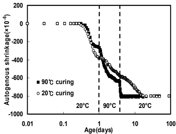
Fig. 3 Effect of curing temperature on the autogenous shrinkage
