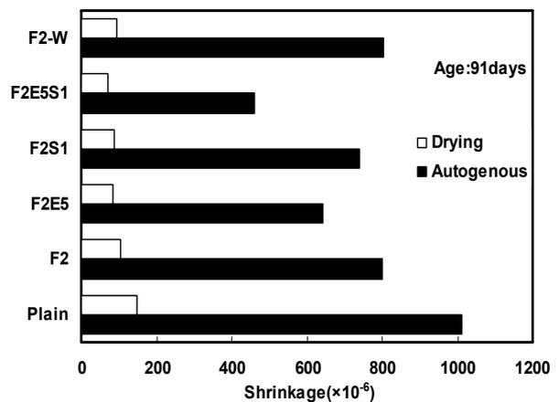
Fig. 9 Comparison of autogenous and drying shrinkages of ultra-high strength SFRC
