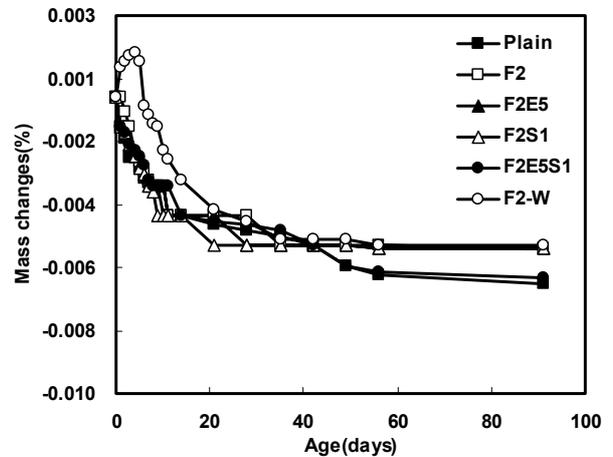
Fig. 8 Mass changes of the specimens during drying shrinkage tests
