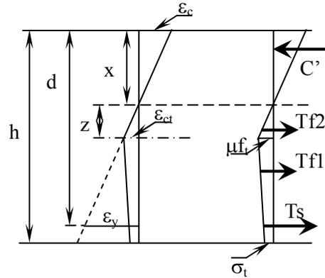
Fig. 6 Strain and stress distribution in SFRC at yielding stage
