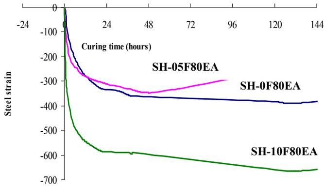
Fig. 5 Steel strain history at mid-span for the case of shear
