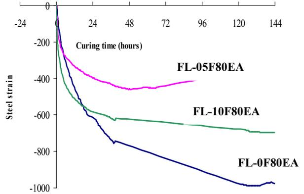
Fig. 4 Steel strain history at mid-span for the case of flexure
