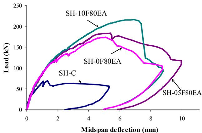
Fig. 8 Load-displacement curve in case of shear
