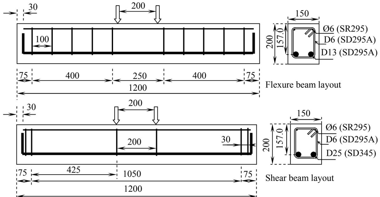
Fig. 2 Beam sizes and reinforcement layout
