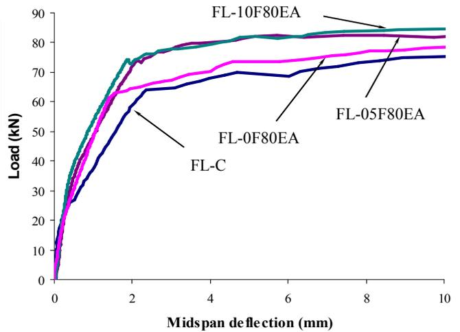
Fig. 7 Load-displacement curve in case of flexure
