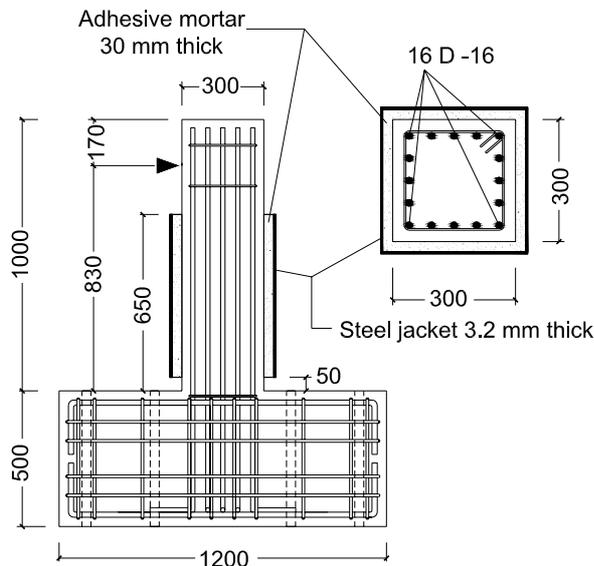
Fig. 1 Details of test specimen
