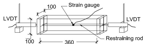
Fig. 2 Details of mould
