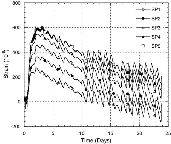
Fig. 3 Strain in restraining rod
