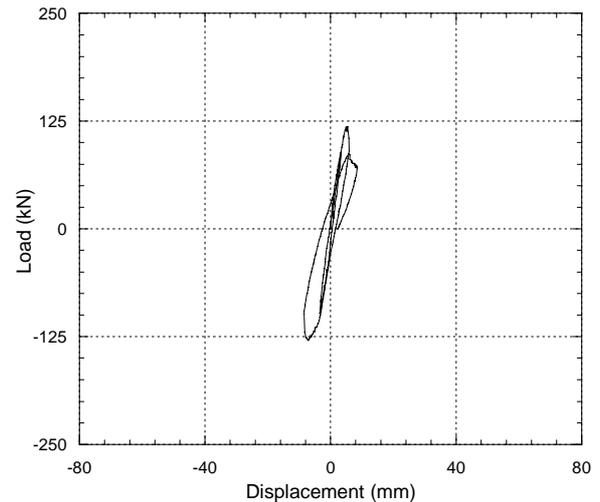
Fig. 7 Load-displacement curve for the control specimen
