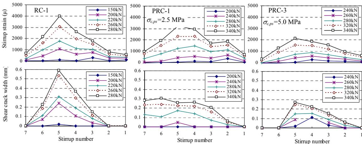
Fig. 5 Variation of shear crack width and stirrup strain along shear span
