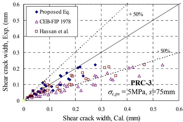
Fig. 8 Accuracy of proposed equation (PRC-3)
