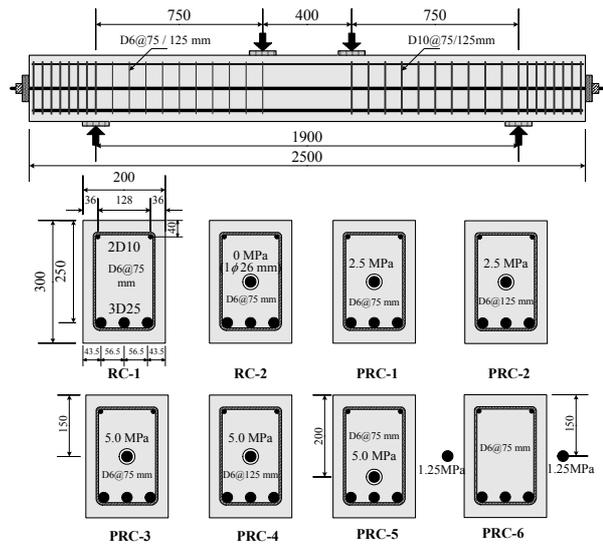
Fig. 3 Typical layout and cross-sectional details of test specimens
