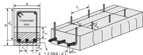
Fig. 2 Parameter influencing crack spacing
