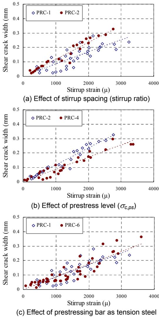
Fig.6 Shear crack width vs. stirrup strain
