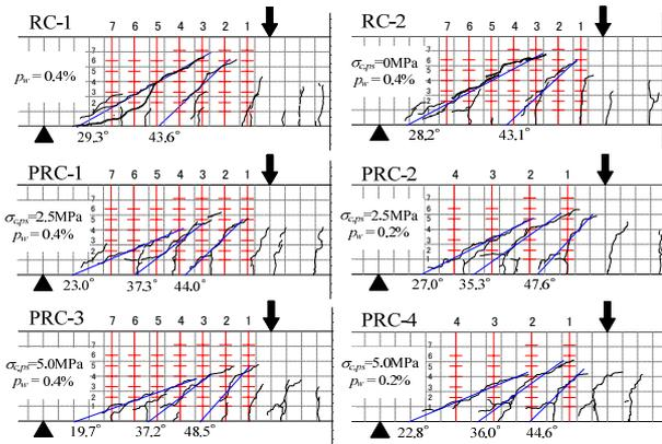
Fig. 4 Crack patterns and crack angles
