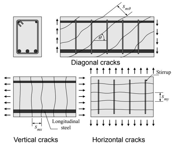
Fig. 1 Modeling of cracks (smeared cracks)
