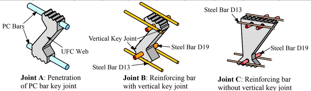
**Fig. 1 Three types of joint method**
