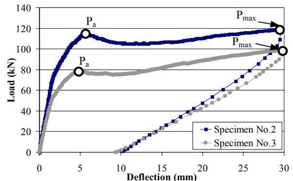
**Fig. 9 Load-deflection curve by comparing the UFC volume of truss member**
