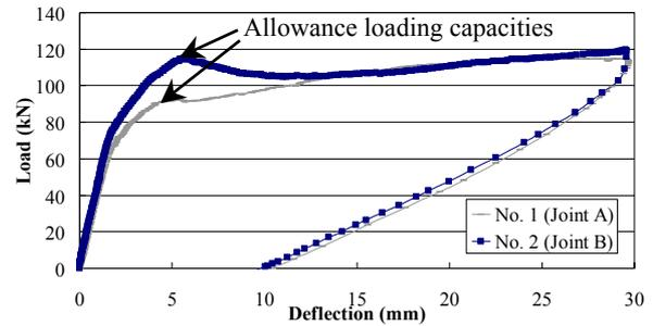
**Fig 4. Load-deflection curve of beams with Joint A and with Joint B**
