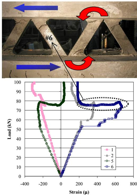
**Fig. 5** UFC truss strain of specimen No.3 (Gauge position shows in Fig. 6)
