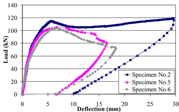
**Fig. 8 Load-deflection curve by comparing the truss member with triangle panel [1]**
