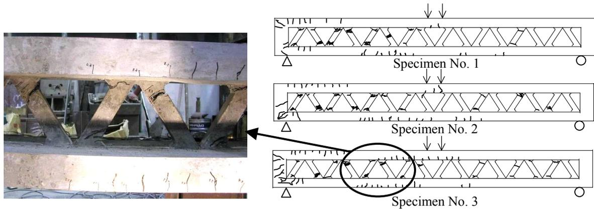
**Fig. 7 Crack patterns of composite PC beams by applying truss as web member**
