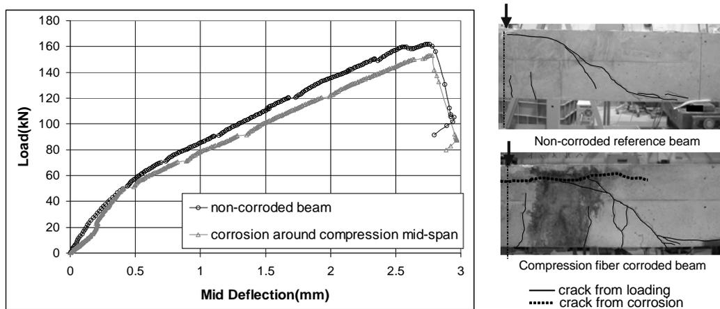
**Figure 3 Load-deflection and failure crack of compression damaged-beam**
