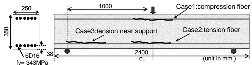
**Figure 1** Specimen details and reinforcement
