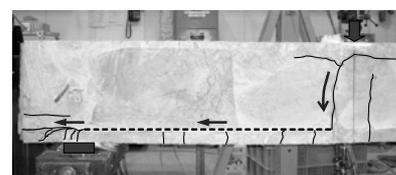
**Figure 8 Inherent crack-like defect over the whole shear span and its elevated capacity (analysis with no anchorage failure) (non-strengthened)**
