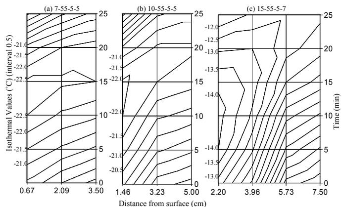
Figure 3 Isotherm chart at minimum temperature during 2nd wet cycle
