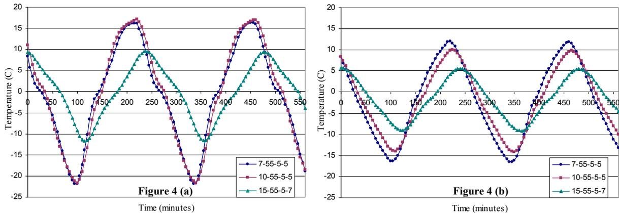
**Figure 4** Typical temperature variations at center of specimens in (a) Wet state, (b) Dry State
