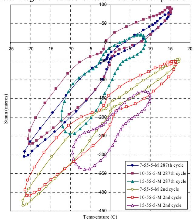
**Figure 5** Strain-temperature curves in wet state
