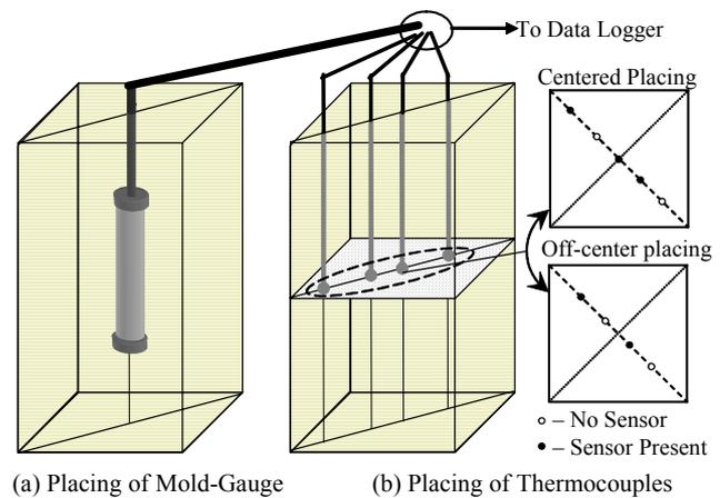
Figure 1 Placing of sensors inside specimens
